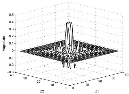
Figure 6: Impulse response of the approximated 2D IIR lowpass filter via VFz.
