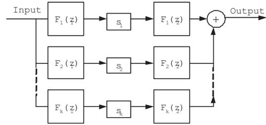
Figure 1: Decomposed FIR prototype filter.
