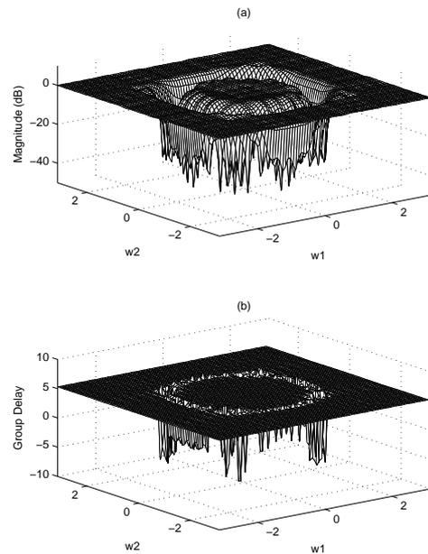
Figure 9: Frequency response of the 2D bandstop IIR filter via the proposed algorithm: (a) magnitude response and (b) group delay in the passband.
