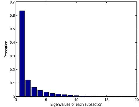
Figure 5: Eigenvalues of the lowpass filter example  $H_1$  of (7) in ratio, which shows the importance of each subsection.
