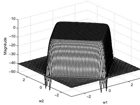
Figure 2: Magnitude response of the 2D prototype low-pass FIR filter by SDP.
