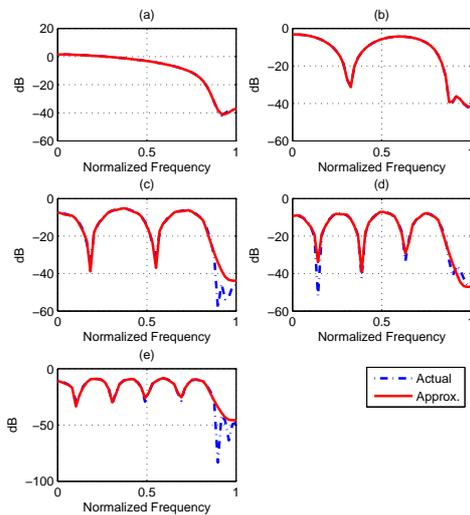
Figure 7: Magnitude response of subfilter approximation using VFz. (a) - (e) are subfilters of sections 1-5 respectively.
