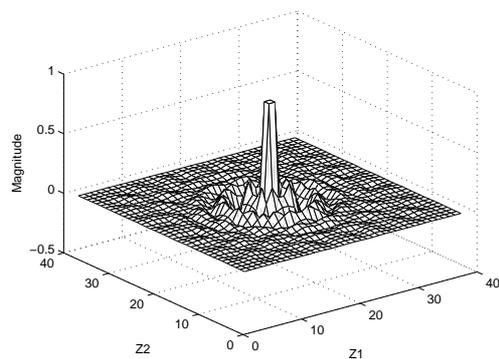
Figure 10: Impulse response of the approximated 2D FIR bandstop filter via VFz.
