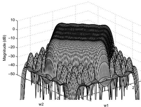
Figure 3: Magnitude response of the approximated 2D lowpass FIR filter after SDM.
