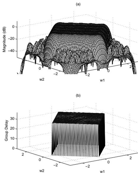
Figure 4: Frequency response of the approximated 2D lowpass IIR filter via VFz: (a) magnitude response and (b) group delay in the passband.
