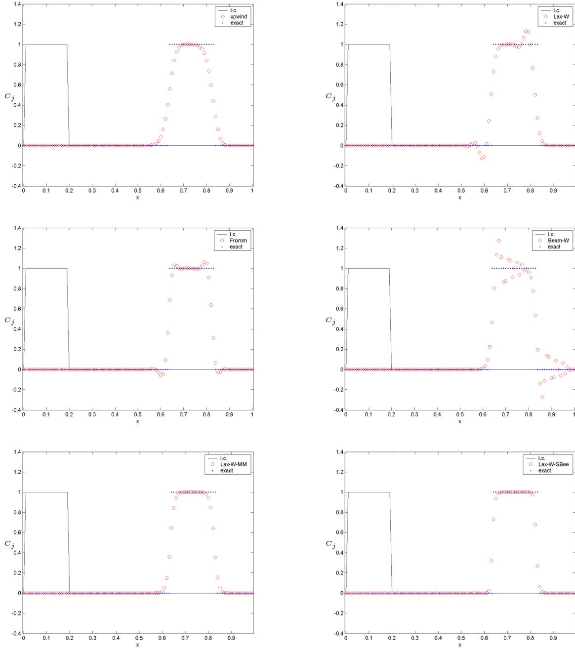
Figure 1: Square initial condition: numerical solutions at  $t = 0.5$  with 100 mesh-cells and  $\nu = .9$ . Top-left: upwind. Top-right: Lax-Wendroff. Middle-left: Fromm. Middle-right: Beam-Warming. Bottom-left: Lax-Wendroff with MinMod limiter. Bottom-right: Lax-Wendroff with Superbee limiter.
