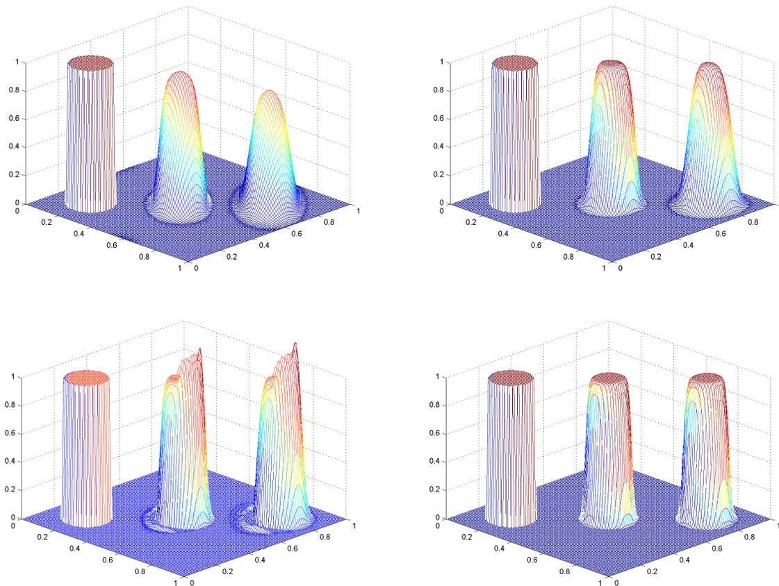
Figure 2: Advection equation with  $100 \times 100$  spatial grid,  $\nu_1 = \nu_2 = 0.95$  and final time  $t_{\max} = 0.6$ . Top left: first order DTU method; top right: first order CTU method; bottom Left: second order Lax-Wendroff method without limiter; bottom right: second order Lax-Wendroff method with van Leer limiter.
