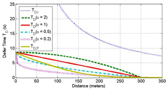
Fig. 1. Different defer times  $T_D$ : the inverse defer time  $T_{D,I}$  in (2),  $T_D$  in (1) with  $\epsilon = 2, 1, 0.5$ , and  $0.2$ , the probabilistic-channel defer time  $T_{D,P}$  in (3)
