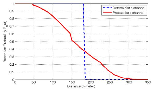
Fig. 4. Packet reception probabilities for the deterministic and probabilistic channels.
