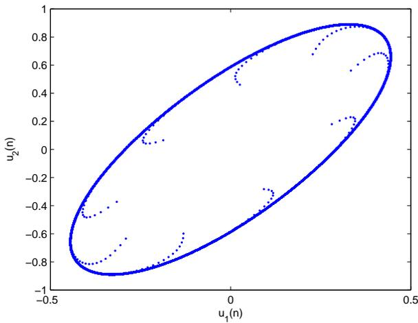
Fig. 2. Dynamical behavior of system (35) with  $\gamma_1 = 0.23$  and  $\gamma_2 = 0.31$ .
