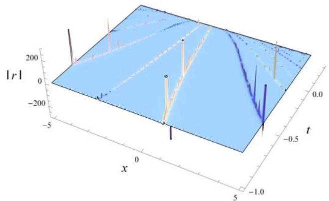
Fig. 6. Spatial structure of bright and dark two-soliton determined by solution (84).
