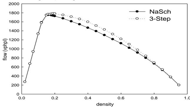
Fig. 1. Flow-density relation of the NaSch and 3-step models for single-lane traffic.
