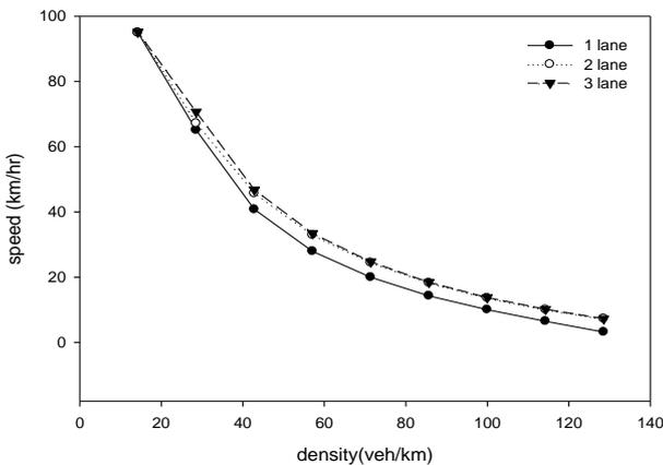
Fig. 2 Speed-density curve of  $v_{max}=4$  and  $p=0.2$ .
