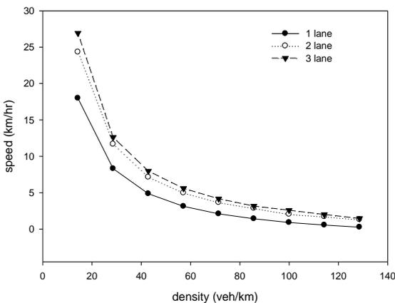
Fig. 3 Speed-density curve of  $v_{max}=4$  and  $p=0.9$ .
