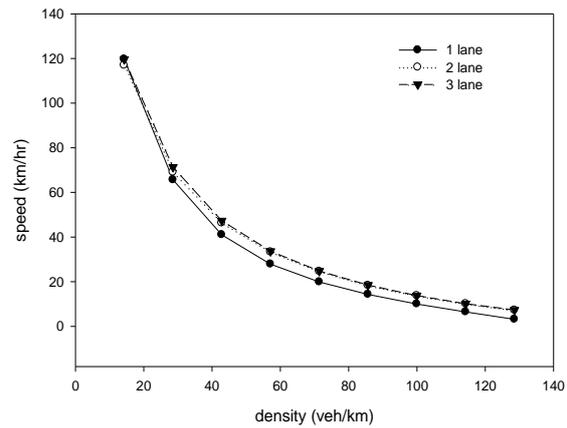
Fig. 4 Speed-density curve of  $v_{max}=5$  and  $p=0.2$ .
