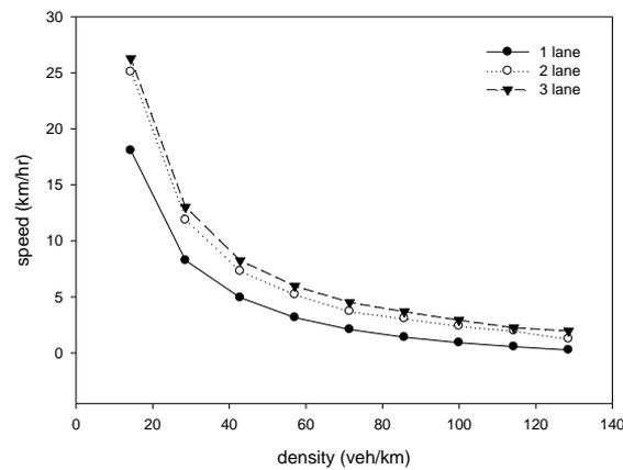
Fig. 5 Speed-density curve of  $v_{max}=5$  and  $p=0.9$ .
