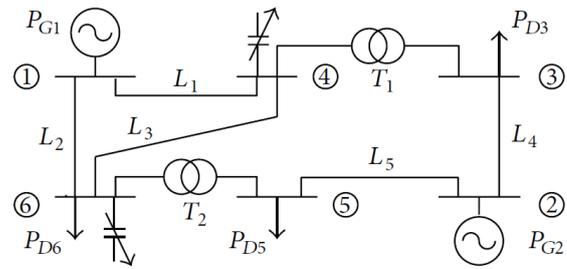
Fig. 6. ESGD Bus Power System from Zhang and Cai [29]
