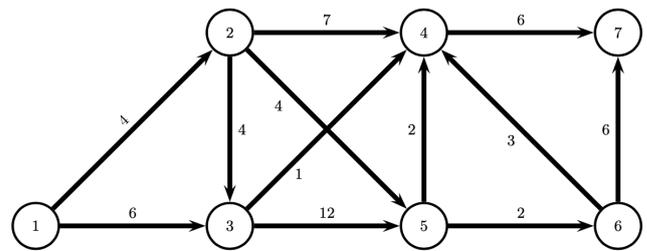
Fig. 2. A maximum flow problem with the nominal arc capacities
