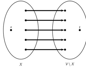
Fig. 1.  $s - t$  cut determined by node set  $X$
