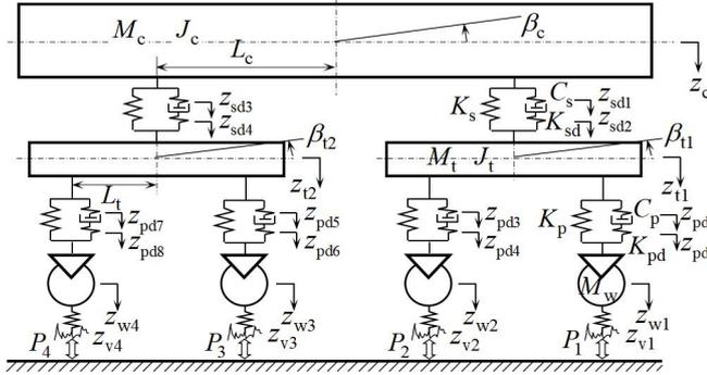
Fig. 1. Traditional railway vehicle vertical dynamic model
