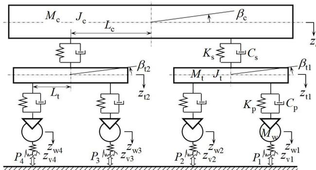
Fig. 2. Railway vehicle vertical dynamic model under the effect of damper rubber joint stiffness
