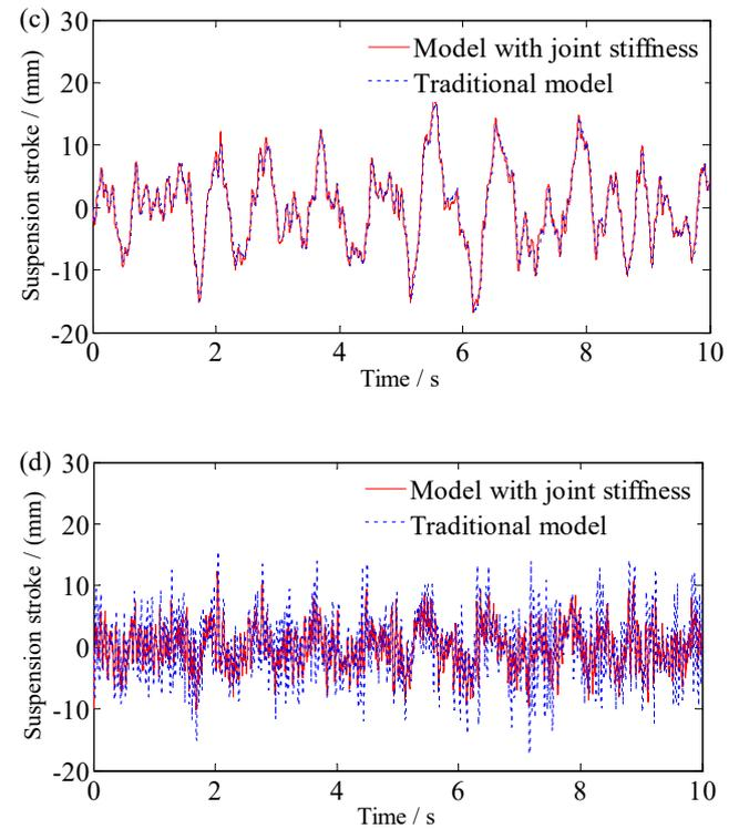
Fig. 4. Analysis results: (a) the car body acceleration; (b) the bogie frame acceleration; (c) the secondary suspension stroke; (d) the primary suspension stroke
