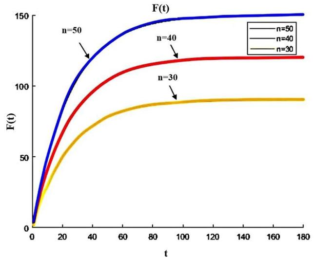
Fig. 2. The volume fraction of exhaled air when number of students are static.
