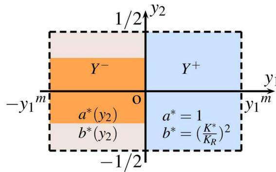
Fig. 12. The domain  $\mathbf{Y} = Y^- \cup Y^+$ , with  $Y^- = (-y_1^m, 0) \times Y_2, Y^+ = (0, +y_1^m) \times Y_2$ .  $\tilde{a}^*(\mathbf{y}) = a^*(y_2)$  and  $\tilde{b}^*(\mathbf{y}) = b^*(y_2)$  in  $Y^-$ , and  $a = 1, b = (\frac{K^*}{K_R})^2$  in  $Y^+$
