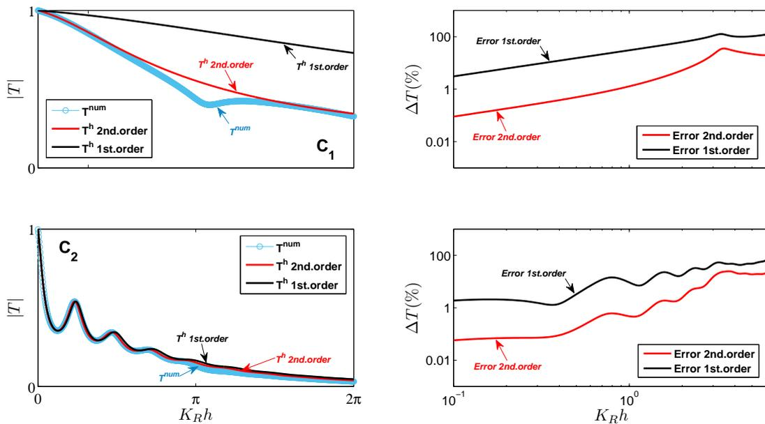
Fig. 7. Left: Transmission coefficients  $|T^{num}|$  and  $|T|$  as a function of  $K_R h$  for  $e/h = 0.05$  and  $e/h = 4$  ( $C_1, C_2$  profiles from Figure 6), with  $|T^{num}|$ : blue symbols and  $|T|$ : black lines at first order and red lines at second order. Right: The corresponding error  $\Delta T$  of the homogenized predictions, which are shown in percent (black lines at first order and red lines at second order).
