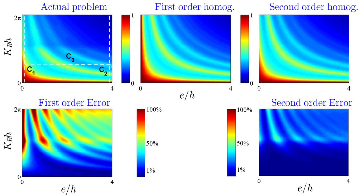
Fig. 6. Up: Transmission coefficients in actual problem  $|T^{num}|$  and homogenized  $|T|$  at first order ( $B = C = 0$ ), and at second order as a function of  $e/h$  and of the frequency  $K_R h$ ; ( $Q^{-1} = 0.2$ ,  $\varphi = 0.1$ ,  $\theta = \pi/3$  and  $\gamma = \pi/6$ ) have been considered. Down: Errors  $\Delta T$  on the transmission coefficient, which are calculated numerically. Errors smaller than 1% appear in dark blue, and errors greater than 100% appear in dark red.
