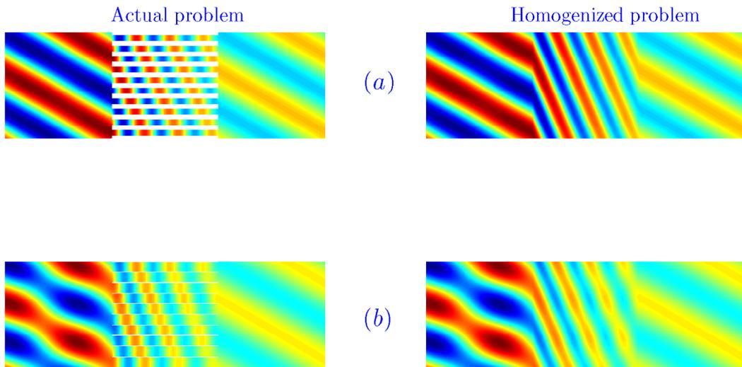
Fig. 5. (a) Same representation as in Figure 4 with the reciprocal quality factor  $Q_{in}^{-1} = 0.1$  for viscoelastic layers of rectangular voids  $\Omega_s$  and  $Q_m^{-1} = 0$  for elastic substrate. (b) Same representation as (a) with  $\varphi = 0.9$ .
