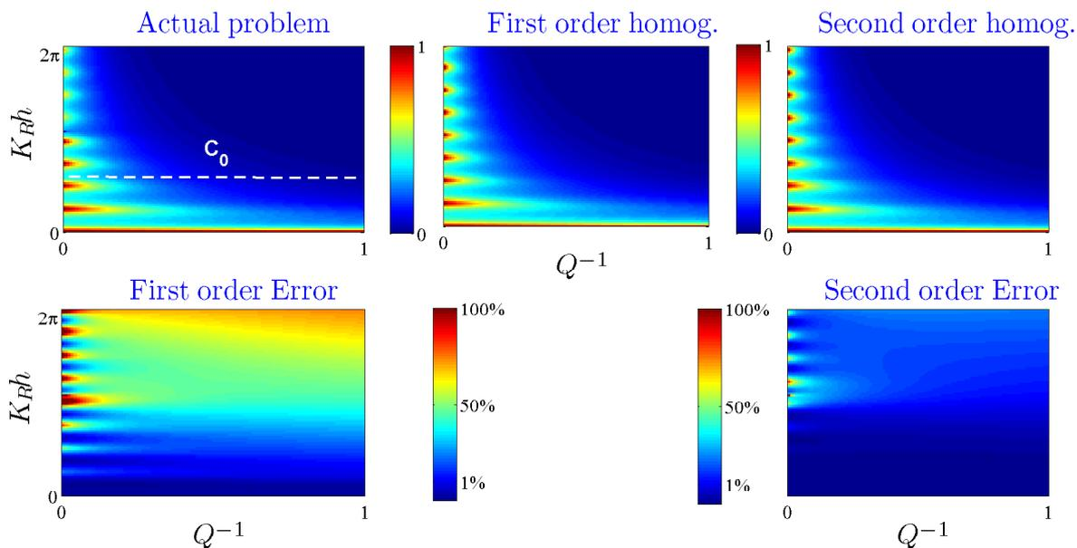
Fig. 9. Up: Transmission coefficients in actual problem  $|T^{num}|$  and homogenized  $|T|$  at first order ( $B = C = 0$ ), and at second order as a function of  $Q^{-1}$  and of the frequency  $K_R h$ ; with  $(e/h = 4, \varphi = 0.1, \theta = \pi/3$  and  $\gamma = \pi/6)$ . Down: Errors  $\Delta T$  on the transmission coefficient, which are calculated numerically. Errors smaller than 1% appear in dark blue, and errors greater than 100% appear in dark red.
