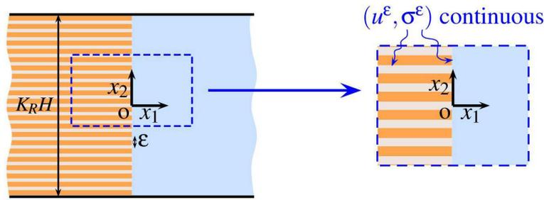
Fig. 2. Single interface between the stratified medium occupying the region  $x_1 < 0$  and the substrate occupying the region  $x_1 > 0$ . The usual continuity conditions apply at the boundaries between the layers  $(u^\epsilon, \sigma^\epsilon)$  and at the boundaries between the layers and the substrate  $(u^\epsilon, \sigma_1^\epsilon)$  at  $x_1 = 0$ .
