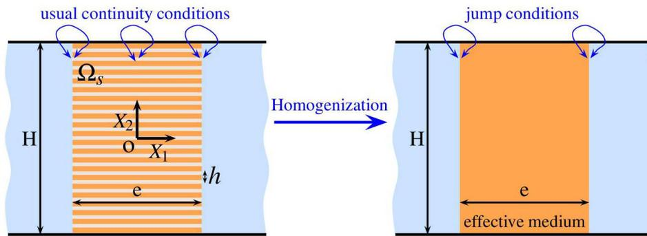
Fig. 1. On the left, the actual configuration of a viscoelastic body (in blue) with a viscoelastic stratified medium  $\Omega_s = \{(X_1, X_2) \in (-e/2, e/2) \times (-H/2, H/2)\}$ . On the right, the homogenized configuration where the stratified medium is replaced by an equivalent homogeneous anisotropic slab, which associated with jump conditions apply at the boundaries of the slab.
