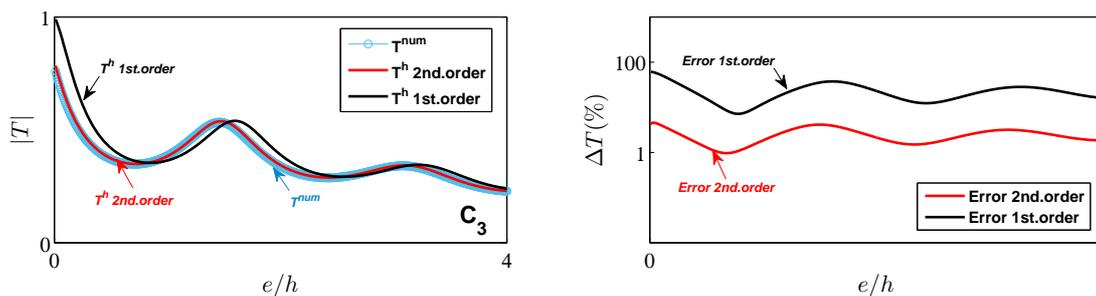
Fig. 8. Transmission coefficients  $|T^{num}|$  and  $|T|$  and errors  $\Delta T$  as a function of  $e/h$  for  $K_R h = 0.6\pi$  ( $C_3$  profile from Figure 6). Same representation as in Figure 7.
