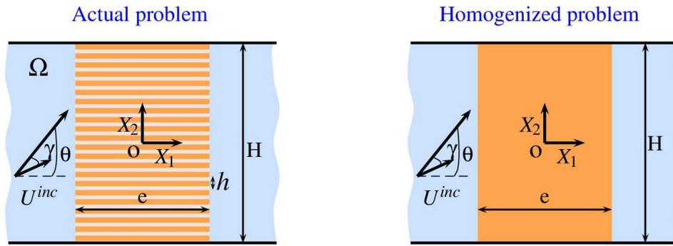
Fig. 3. Left: Actual problem of the scattering of a plane wave at oblique incidence  $\theta$  of an array of rectangular voids, with degree of heterogeneity  $\gamma$ . Right : The homogenized problem involves a slab of same thickness  $e$  filled with a homogeneous anisotropic material, which associated with jump conditions and apply at  $X_1 = \pm e/2$ .
