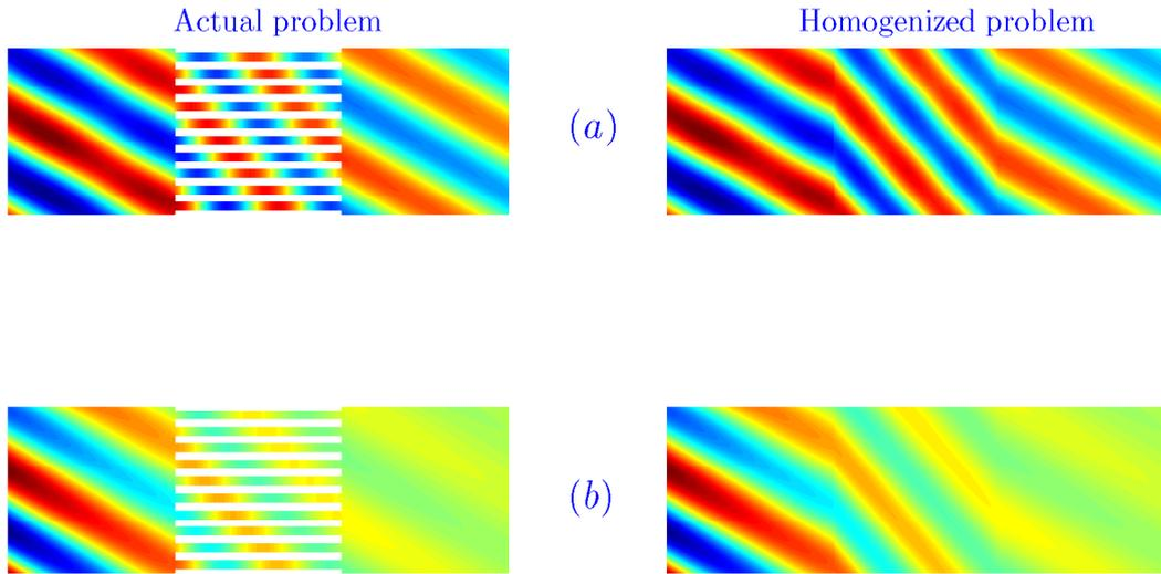
Fig. 4. (a) The numerical solution  $U^{num}$  in the actual problem of low-loss viscoelastic media ( $Q^{-1} = 0.05$ ), for an oblique incident plane wave  $\theta = \pi/3$  with degree of heterogeneity  $\gamma = \pi/6$  and  $K_R h = 1$  on an array made of rectangular voids ( $e/h = 10$  and  $\varphi = 0.5$ ); the right shows the homogenized fields  $U$ . (b) Same representation as (a) with  $Q^{-1} = 0.2$  in the case of low-loss viscoelastic media.
