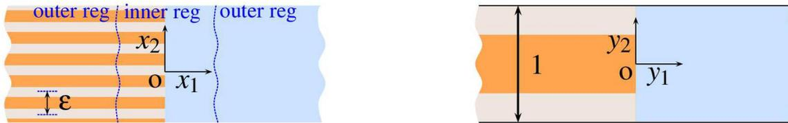
Fig. 11. Left: configuration in the  $x$  coordinate; the periodicity along  $x_2$  is  $\varepsilon \equiv K_R h$ ; the inner region corresponds to the neighborhood of the boundary between the stratified medium ( $x_1 < 0$ ) and the substrate being a homogeneous medium ( $x_1 > 0$ ). Right: the unit cell (inner region) in the  $y$  coordinate, with  $\mathbf{y} = \mathbf{x}/\varepsilon$ , and  $\mathbf{y} \in \mathbb{R} \times Y_2$ , with  $Y_2 = (-1/2, 1/2)$ .
