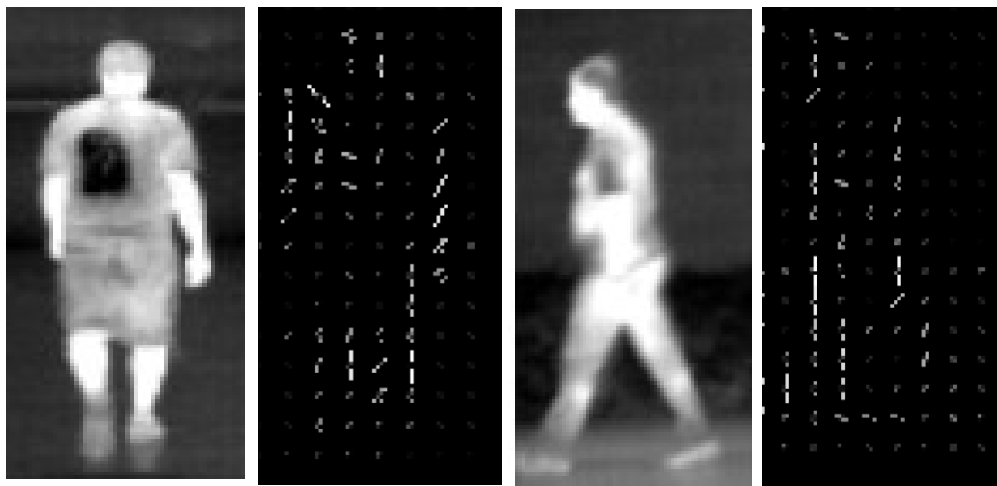
Fig. 3. Two pedestrian images with corresponding HOG feature images
