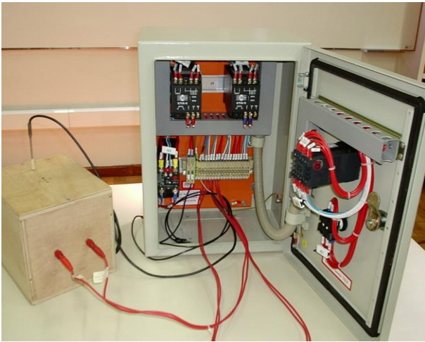
Fig. 2. Temperature Control System.
