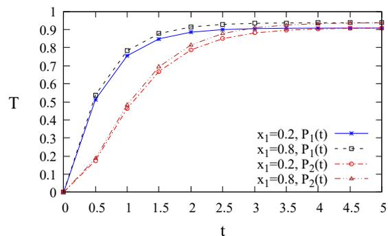
Fig. 7. Solution  $T$  at points  $(0.2, 0.5), (0.8, 0.5)$  for Problem 2 of isotropic inhomogeneous material.
