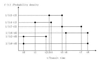
Fig. 2. Diagram of transit time distribution under different situations
