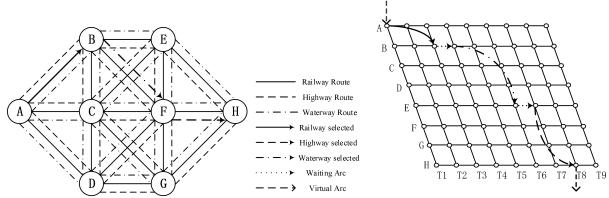
Fig. 1. Examples of physical network and time-space network
