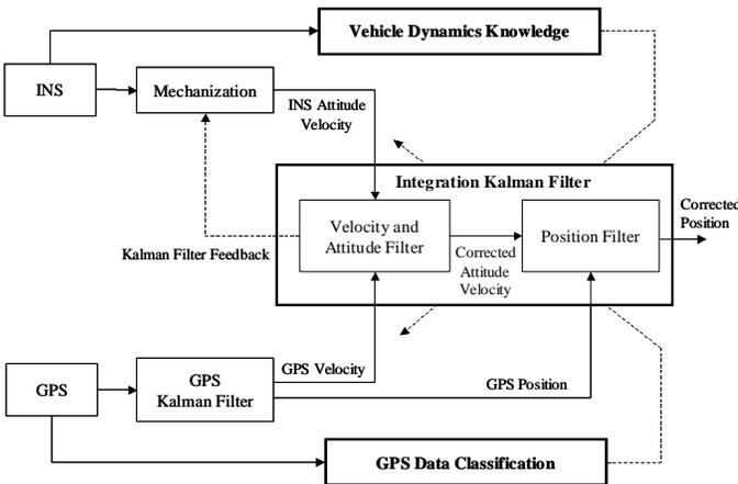
Fig. 3. Architecture of AI-enhanced integration algorithm.
