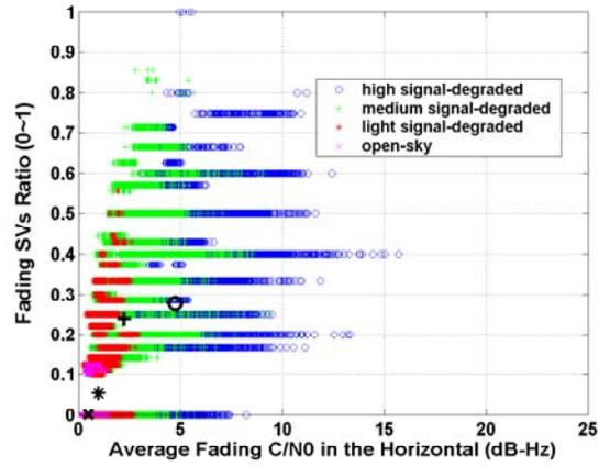
Fig. 1. Distribution of the geo-signal degradation measures in various signal degradation environments.
