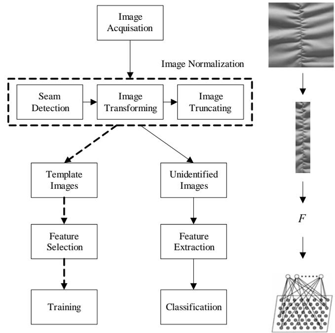
Fig. 3. Block diagram of the classification system.
