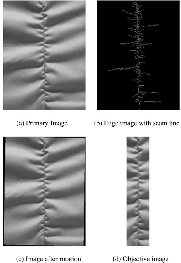
Fig. 4. Seam detection, image transforming and truncating. (a) is the primary gray-level image acquired by a CCD camera system, and (b) is the image after canny edge detection with the seam line positioned by Hough transform. In (c) and (d) are the images after rotation and truncating, respectively.
