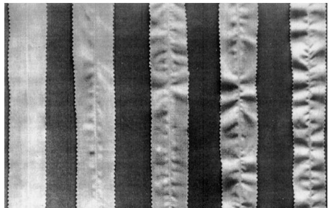
Fig. 1. Photographic standards for subjective pucker inspection by the AATCC method [2].
