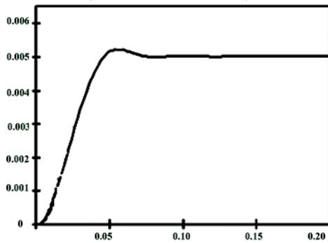
Fig. 15 PD with unit input disturbance (Radians vs. Seconds)
