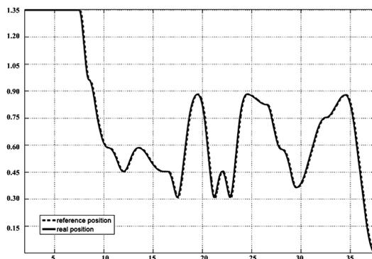
Fig.10. Comparison between planned and followed trajectory of joint1 (Radians vs. Seconds)
