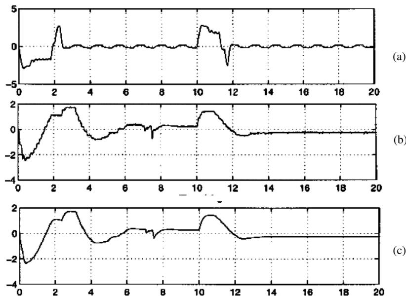
Fig.16.Robot Joint 1 tracking performance (a) FLC implementation, (b) LQR implantation, (c) Slide mode control implementation
