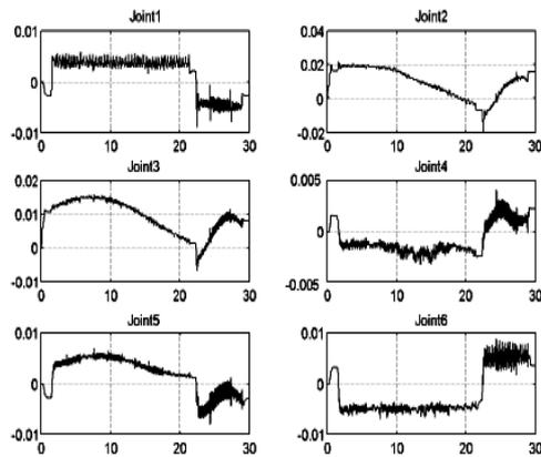
Fig 9 Position tracking error (Radians vs. Seconds)
