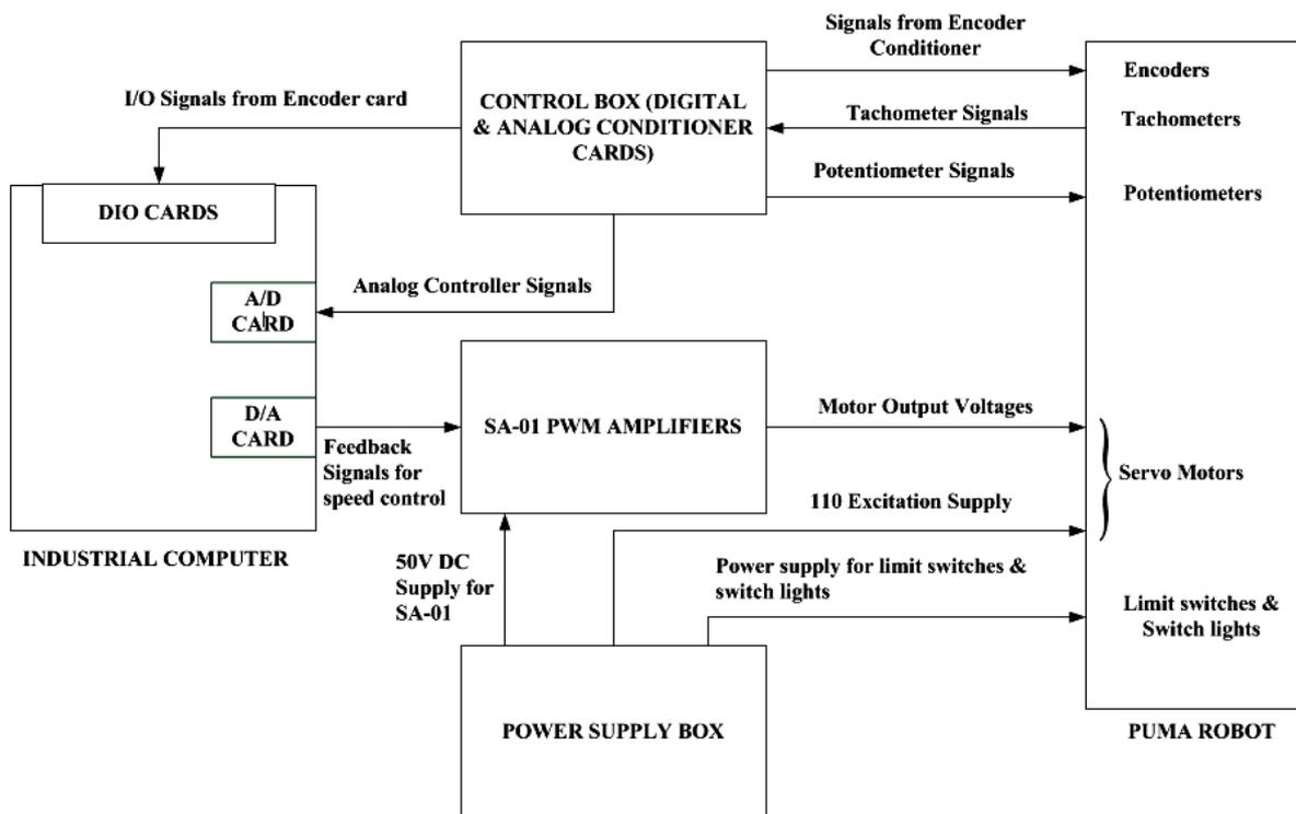
Fig. 3 Schematic diagram of new robot hardware
