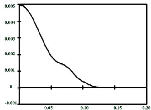
Fig. 12 FLC with friction  $\approx 0.23\text{Nm}$  (Joint1 of robot) (Radians vs. Seconds)
