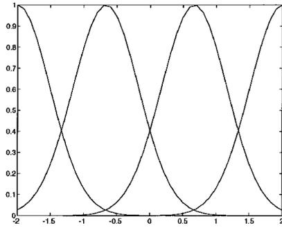
Fig. 5 Membership functions for fuzzy controller with 16 rules.
