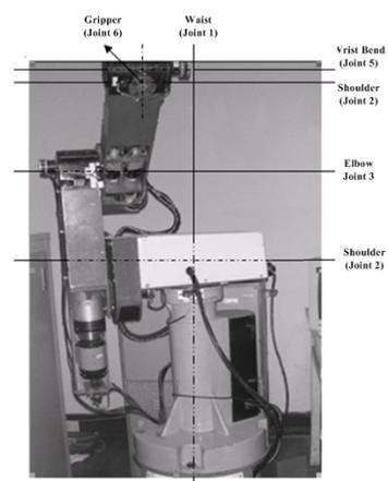
Fig.2 PUMA robot 512 joints identification
