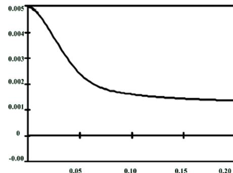
Fig. 13 PD with friction  $\approx 0.23\text{Nm}$  (Joint 1 of robot) (Radians vs. Seconds)
