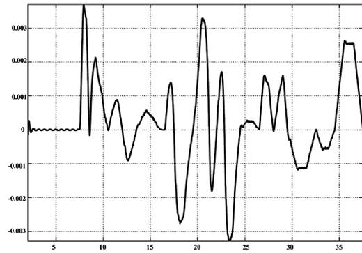
Fig.11 Trajectory tracking error for joint1. (Radians vs. Seconds)
