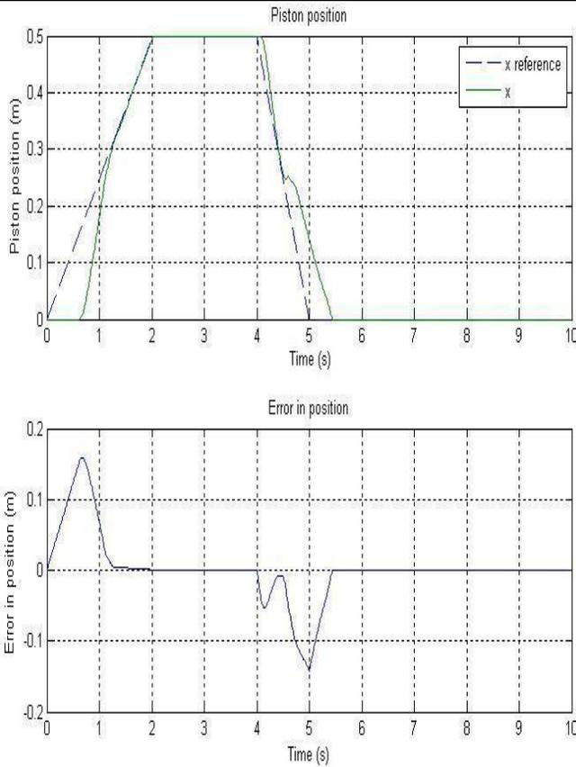
Fig. 6 Closed loop no-load piston position and error in position responses of Neural Network based PI controlled pneumatic system.
