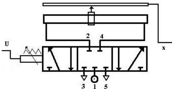
Fig. 1 The Schematic diagram of the servo pneumatic actuator.
