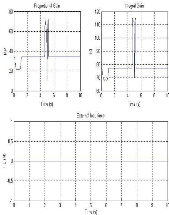
Fig. 7 Closed loop no-load  $K_p$ ,  $K_i$  and  $F_L$  responses of Neural Network based PI controlled pneumatic system.
