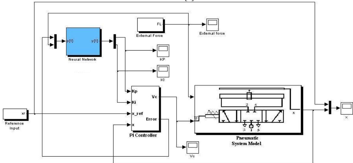
Fig. 4 Block diagram of the Neural Network based intelligent PI controlled pneumatic system.
