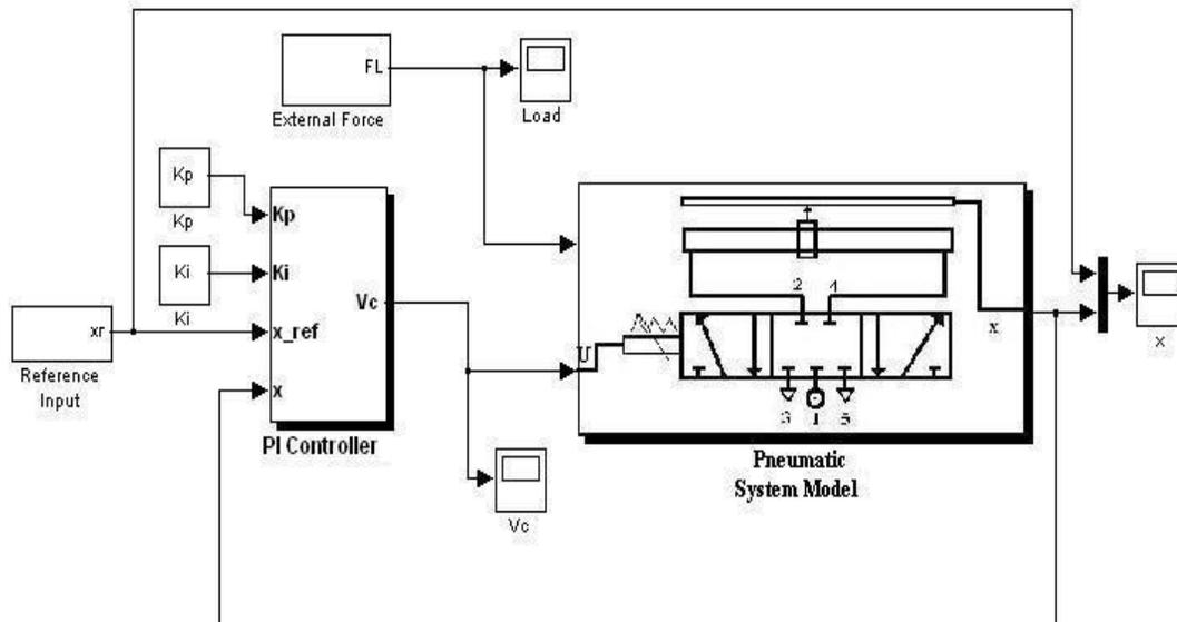
Fig. 3 Closed loop PI controlled pneumatic system.
