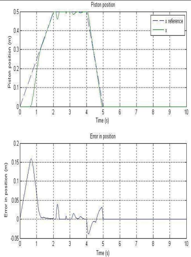
Fig. 8 Closed loop variable-load force piston position and error in position responses of Neural Network based PI controlled pneumatic system.
