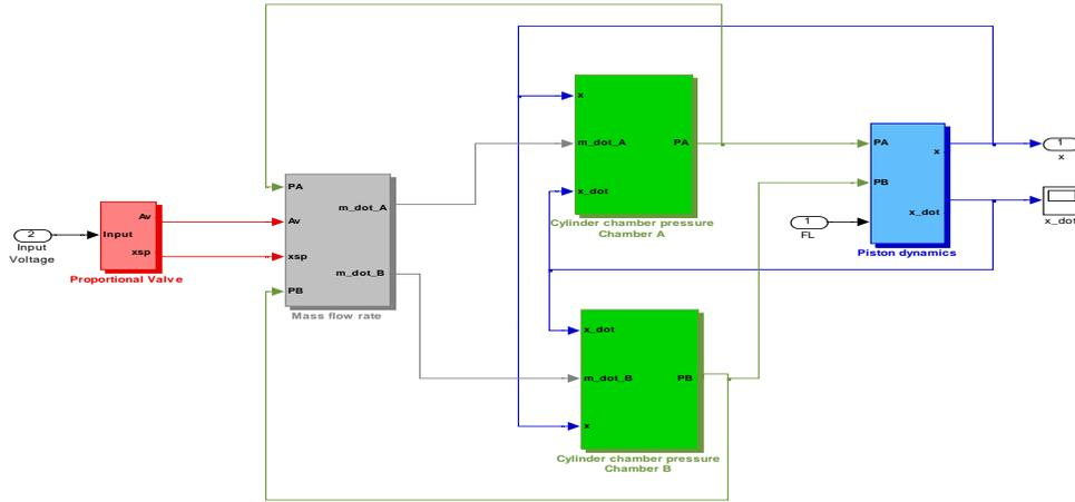
Fig. 2 Simulation model of Nonlinear mathematical model of the servo pneumatic actuator.
