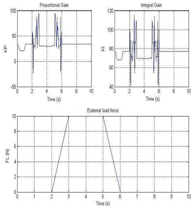
Fig. 9 Closed loop variable-load force  $K_p$ ,  $K_i$  and  $F_L$  responses of Neural Network based PI controlled pneumatic system.
