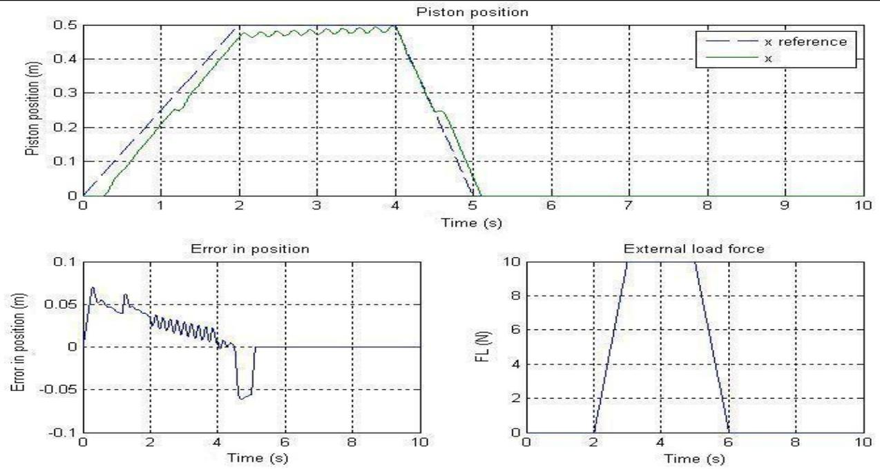
Fig. 10 Closed loop variable-load force responses of PI controlled pneumatic system.
