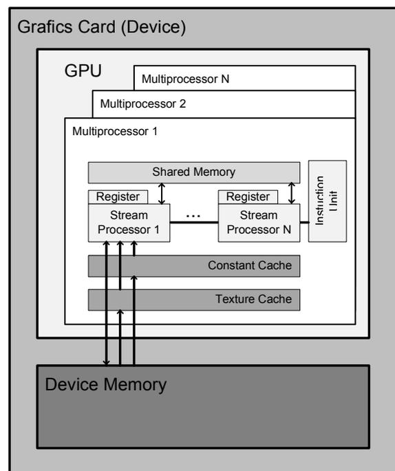
Fig. 3 Block diagram of a graphics card with a GPU and on board memory [7]
