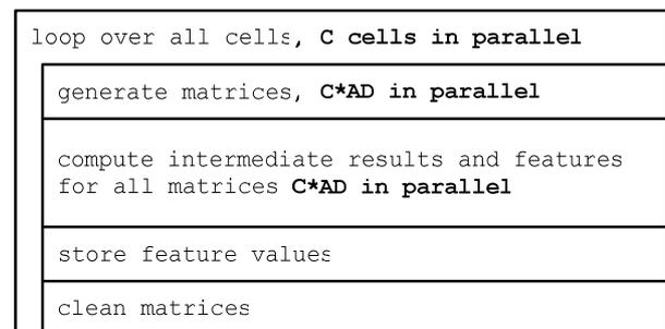
Fig. 9 Structure of the GPU version. Bold marked entries are executed in parallel.
