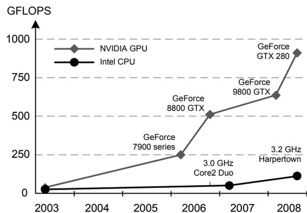
Fig. 2 Peak performance growing curve of different GPU and CPU generations [7]
