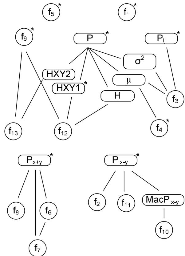
**Fig. 7 The computation dependency graph of the Haralick Texture Features (circles) and intermediate results (boxes). All features and intermediate results marked with an asterisk (\*) depend on the co-occurrence matrices.**
