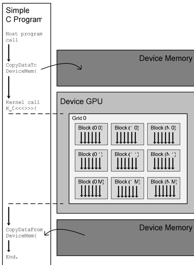
Fig. 4 A simple C program using the GPU [7]
