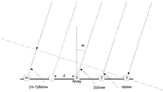
Fig. 1. Arrival delays of wavefront across the array
