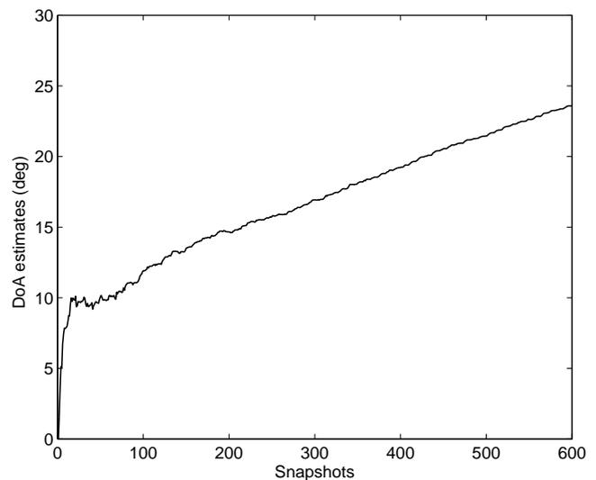
Fig. 5. Results of experiment 4: DOA estimates from a moving source.
