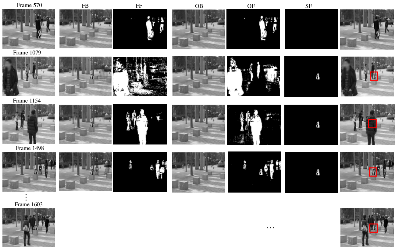
Fig. 10. Detail procedure of abandoned object detection (our own video sequence in outdoor environment).
