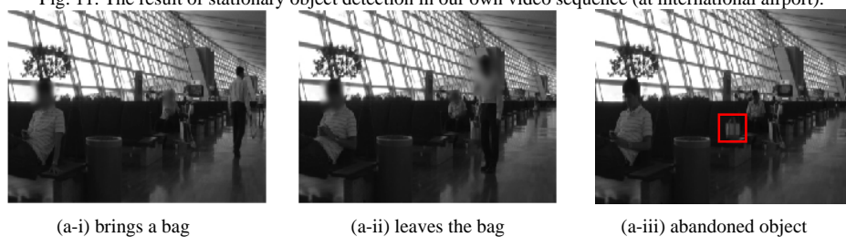
Fig. 11. The result of stationary object detection in our own video sequence (at international airport).
