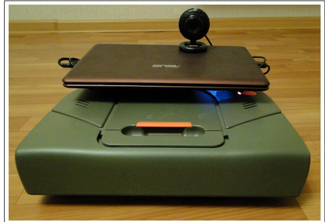
Fig. 3. Robot Neato XV-11 with an onboard computer and a camera.
