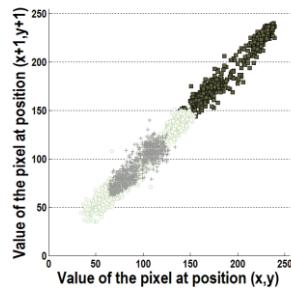
Fig. 7(e). Correlation of vertically adjacent pixels in the original image
