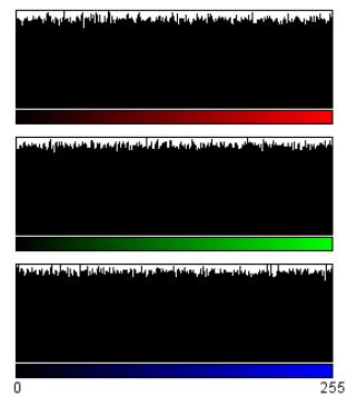
Fig. 6(d). Histogram of the encrypted Lena image
