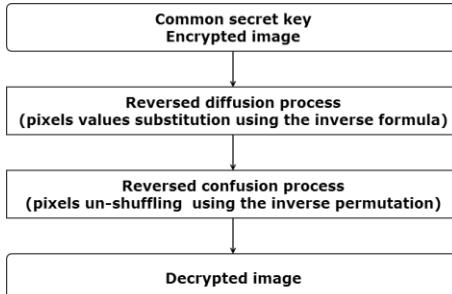
Fig. 2. The block diagram of the decryption process
