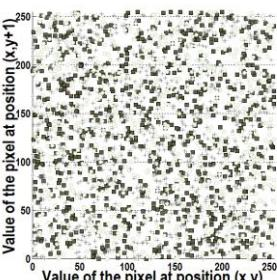
Fig. 7(d). Correlation of vertically adjacent pixels in the encrypted image
