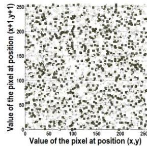
Fig. 7(f). Correlation of vertically adjacent pixels in the encrypted image
