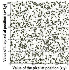
Fig. 7(b). Correlation of horizontally adjacent pixels in the encrypted image
