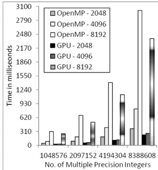
Fig. 2. Binary GCD Using OpenMP and GPU
