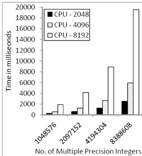
Fig. 7. MBE GCD on CPU
