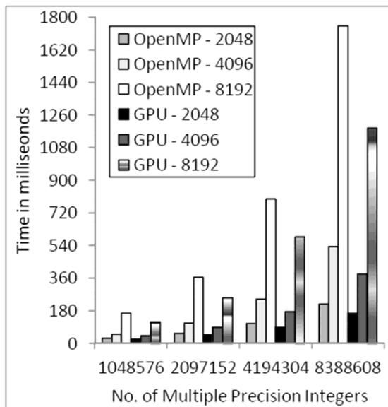
Fig. 8. MBE GCD Using OpenMP and GPU
