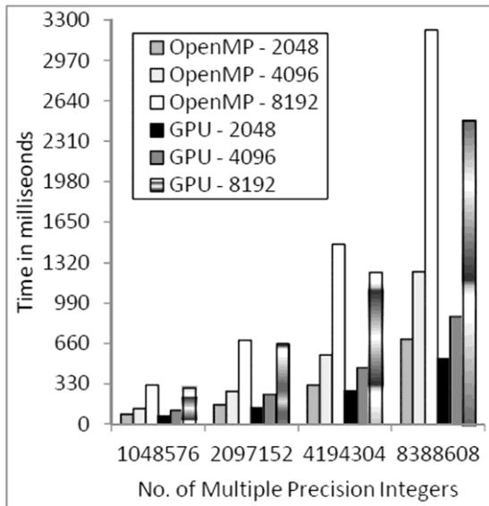
Fig. 6. EEA GCD Using OpenMP and GPU
