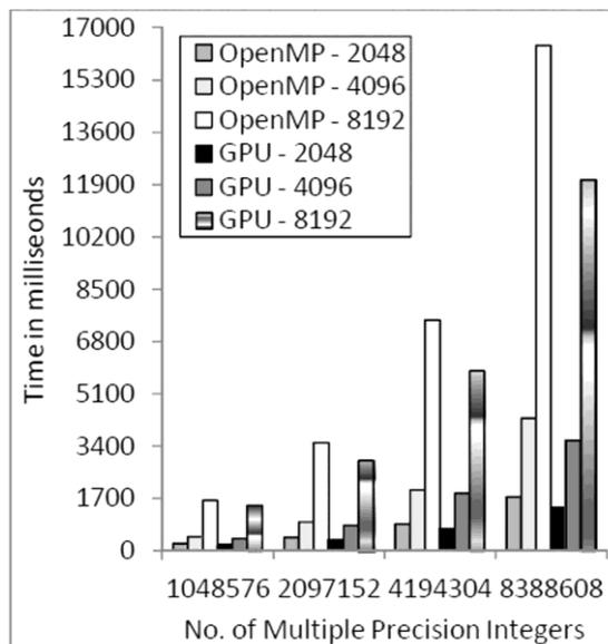
Fig. 4. EBin GCD Using OpenMP and GPU
