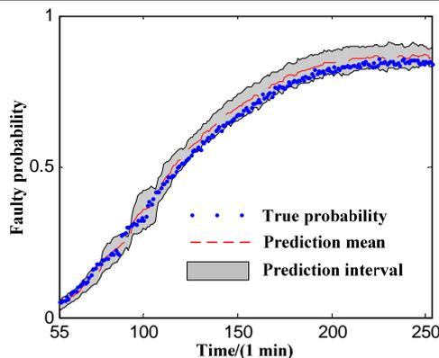
Fig. 10. Faulty probability mean and PI of 5-steps-ahead power prediction by RMRB under gain attenuation failure of intermediate frequency amplifier
