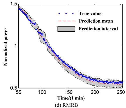
Fig. 8. 5-steps-ahead PIs of gain attenuation failure of intermediate frequency amplifier
