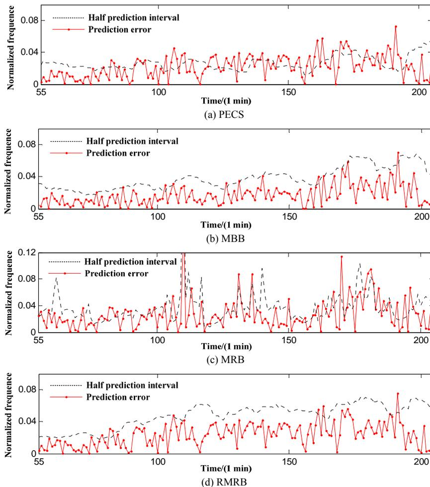
Fig. 6. The absolute value of 5-steps-ahead frequency prediction error and corresponding half PI width under frequency deviation failure of reference-clock.
