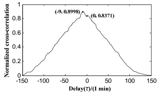
Fig. 2. The normalized cross-correlation between 5-steps-ahead prediction error  $\varepsilon_{k+5}$  and corresponding  $PI_{k+5}$
