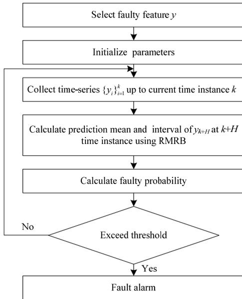
Fig. 1. Fault prediction flow chart
