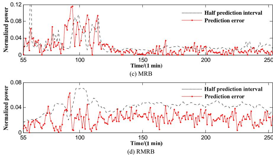
Fig. 9. The absolute value of 5-steps-ahead power prediction error and corresponding half PI width under gain attenuation failure of intermediate frequency amplifier
