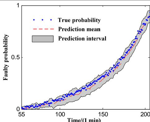
Fig. 7. Faulty probability mean and PI of 5-steps-ahead prediction by RMRB under frequency deviation failure of reference-clock
