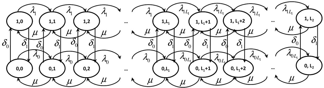
Fig. 4. State transition diagram for system model with Feedback Control
