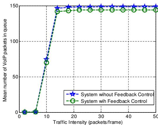
Fig. 6. Mean Number of VoIP Packet in queue under Traffic Intensity.
