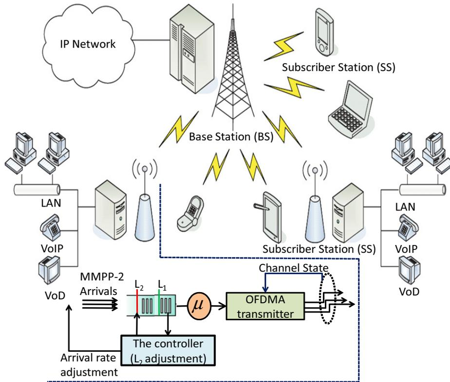
Fig. 2. System model with Feedback Control
