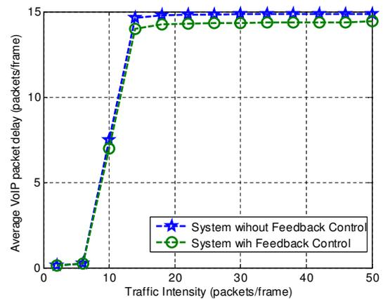
Fig. 7. Average VoIP Packet Delay under Traffic Intensity.
