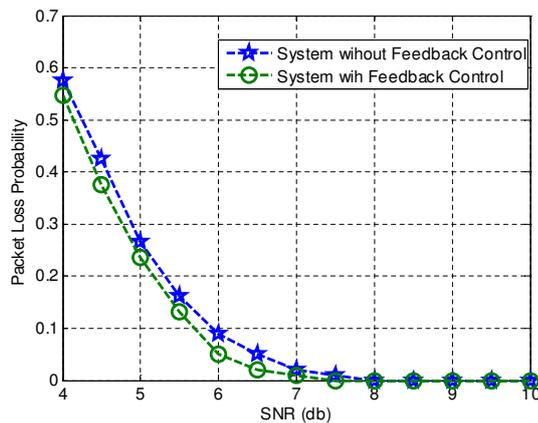
Fig. 9. Packet Loss Probability under different channel qualities.
