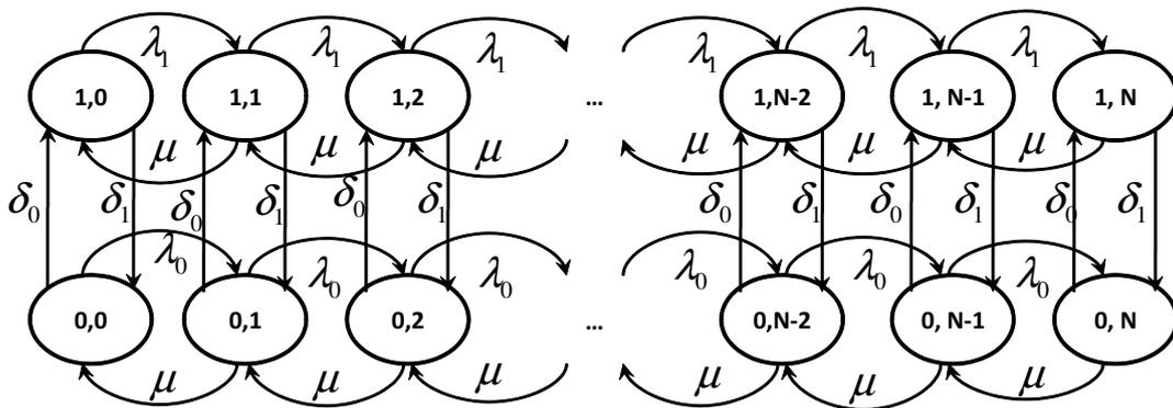
Fig. 3. State transition diagram for system model without Feedback Control
