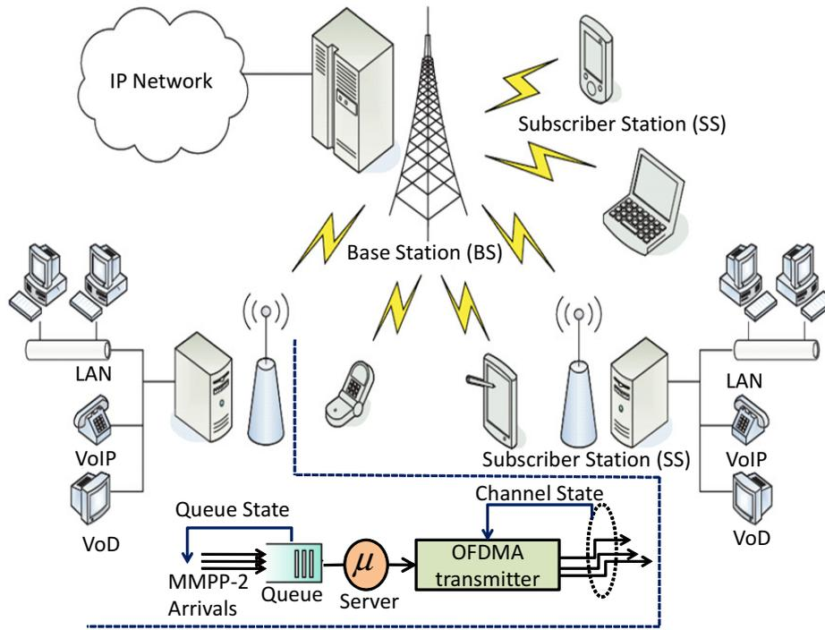
Fig. 1. System model without Feedback Control.
