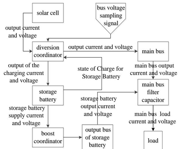
Fig. 1 The schematic structure of satellite power system
