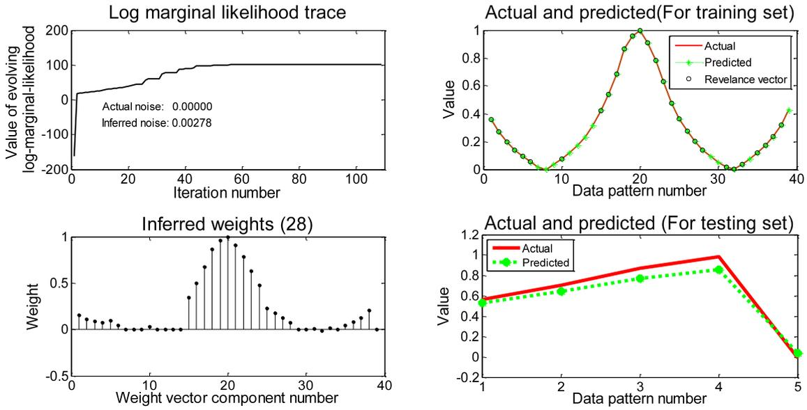
Fig. 4 Inferred weights and forecasting performance when  $\sigma=0.1$
