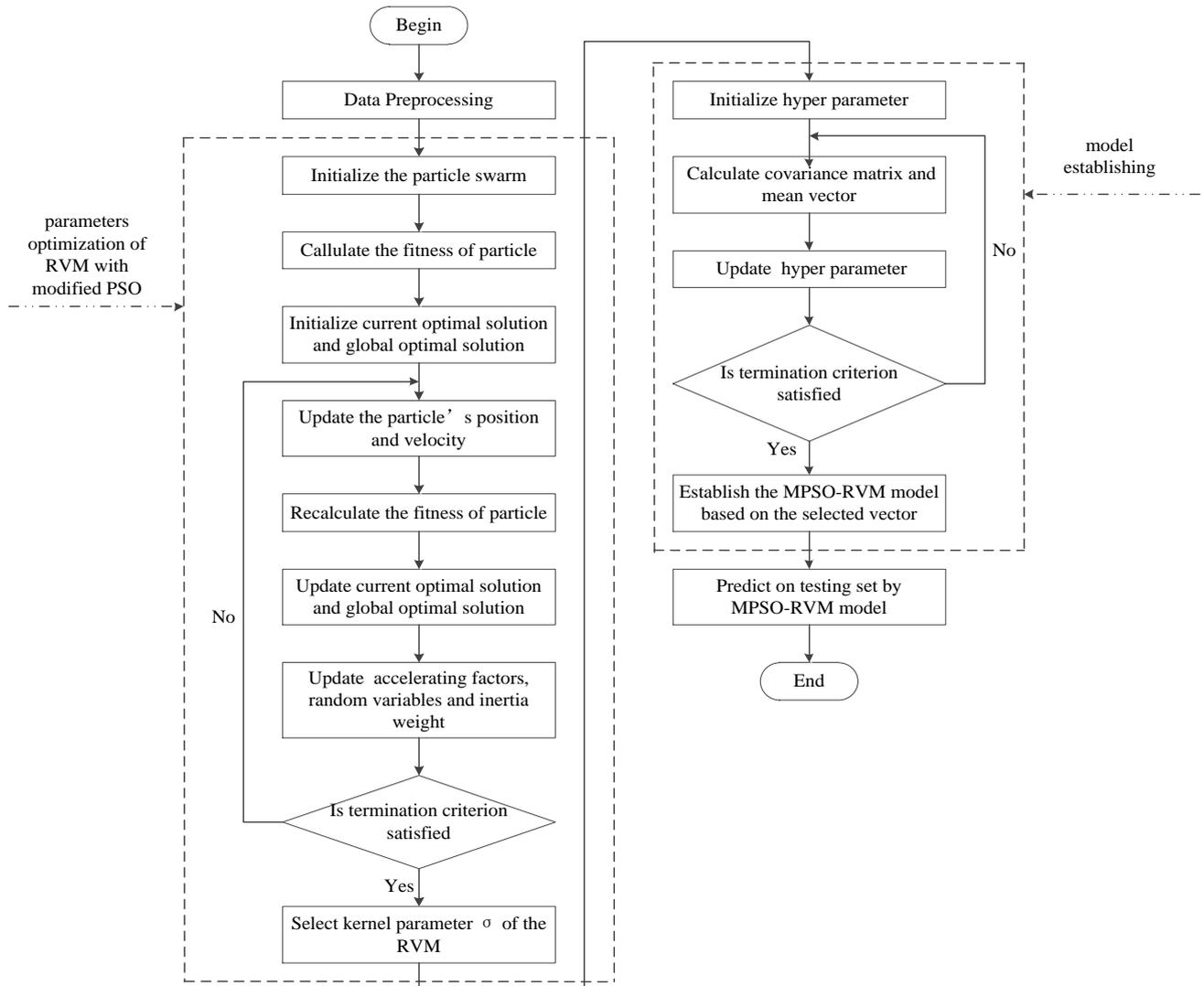
Fig. 2 The flow chart of MPSO-RVM.
