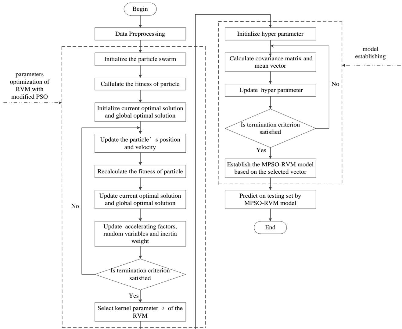
Fig. 2 The flow chart of MPSO-RVM.
