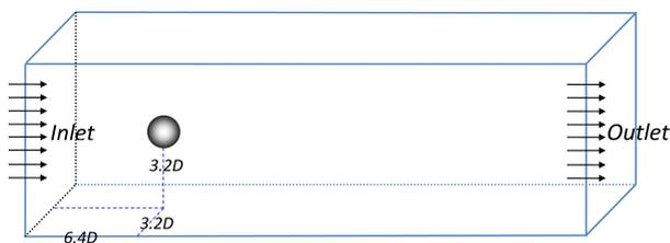
Fig. 17. Flow geometry, coordinate system, and computational domain
