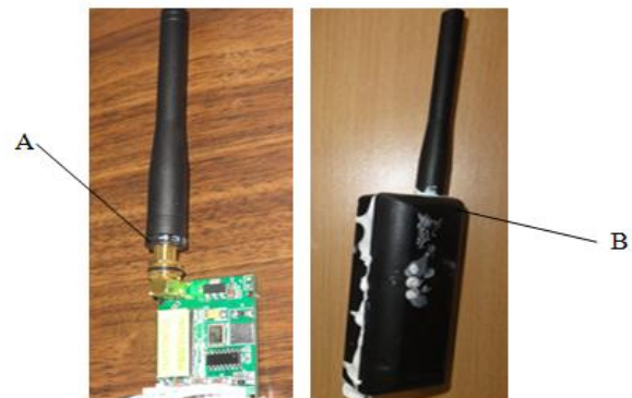
A. Unsealed sensor node B. sealed sensor node Fig.1. Picture of wireless underground sensor network node
