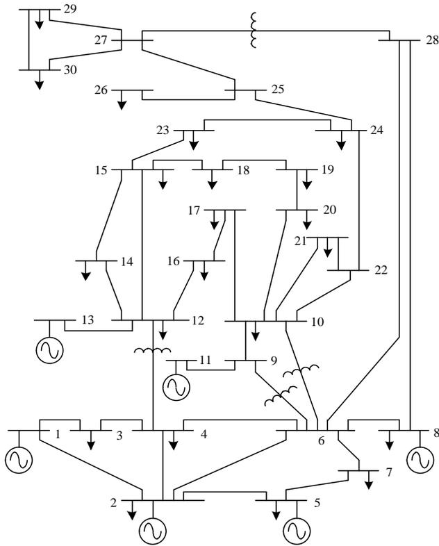
Fig. 1. The system structure diagram of IEEE 30-bus system.
