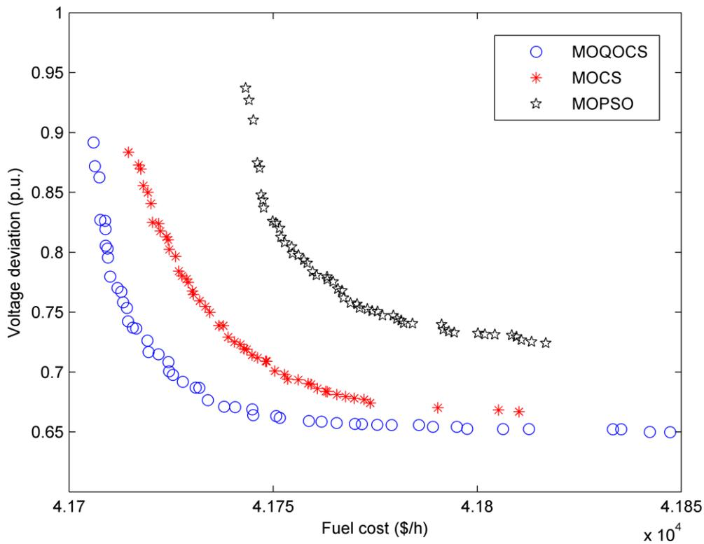
Fig. 6. Pareto optimal fronts of MOQOCS, MOCS and MOPSO for Case 2 of IEEE 57-bus system.
