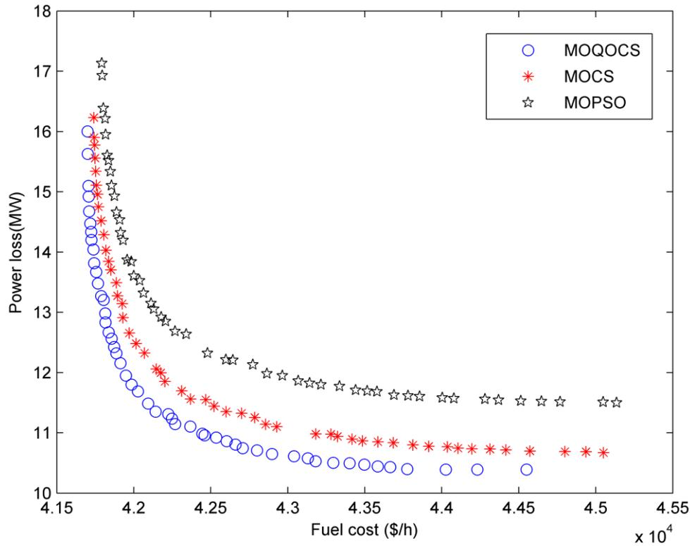
Fig. 5. Pareto optimal fronts of MOQOCS, MOCS and MOPSO for Case 1 of IEEE 57-bus system.
