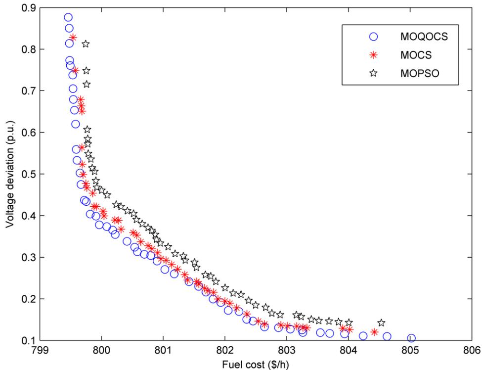
Fig. 3. Pareto optimal fronts of MOQOCS, MOCS and MOPSO for Case 2 of the IEEE 30-bus system.
