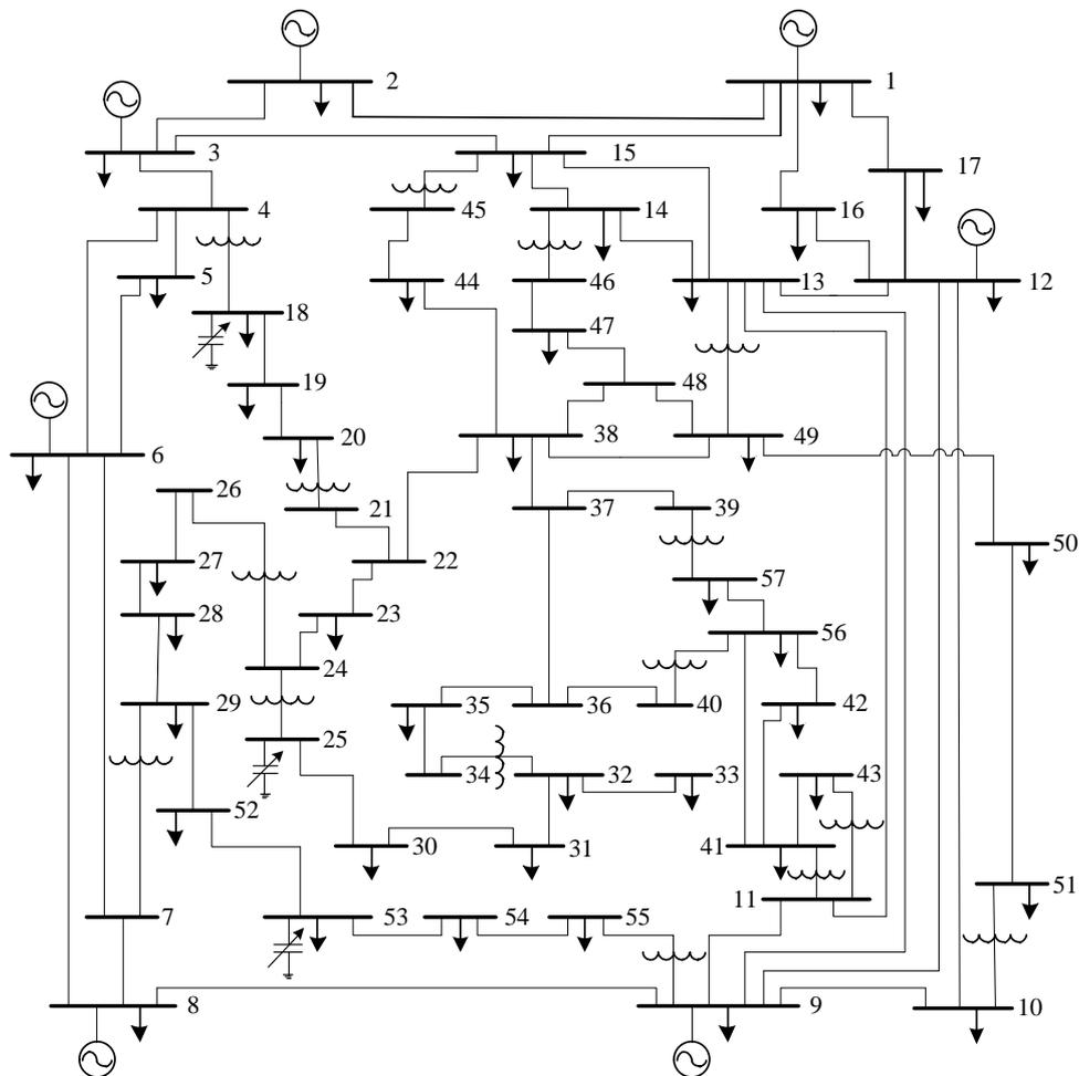
Fig. 4. The system structure diagram of IEEE 57-bus system.
