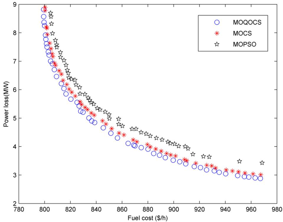
Fig. 2. Pareto optimal fronts of MOQOCS, MOCS and MOPSO for Case 1 of the IEEE 30-bus system.
