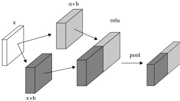
Fig. 1: The original architecture of max-min pooling method for exploiting either positive and negative output of convolution process (adapted from [22]).
