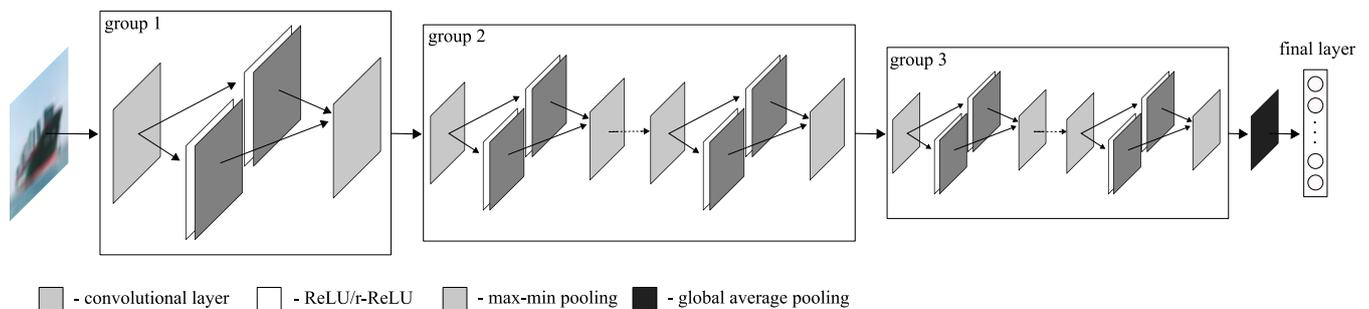
Fig. 5: The CNN structure of the final proposed classifier, which is a modification of net-E network configuration (please see Table I). The detail configuration of each layer can be viewed in Table IV.
