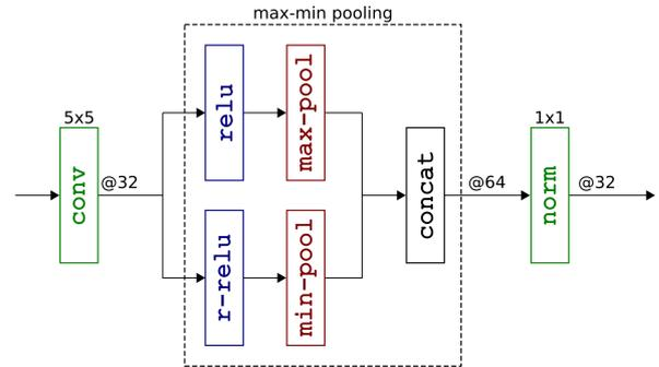
Fig. 2: The proposed extended max-min pooling to reduce the number of parameters by adding normalization layer at the end of the module. The diagram assumed that convolution kernel has 32 channel output.
