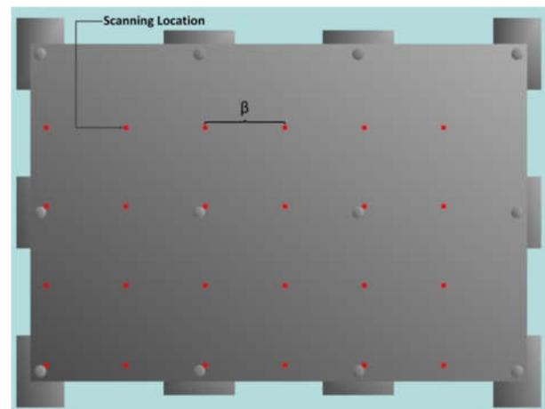
Figure 4. 24 potential scanning locations are generated for the example of the simple structure of Figure 4, using  $\beta=2m$
