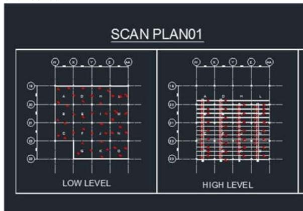
Figure 1. Low-level and high-level scanning plan generated manually by a professional surveyor
