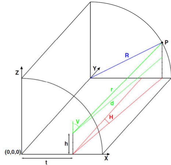
Figure 2. Diagram depicting measurement of a circular tunnel using TLS
