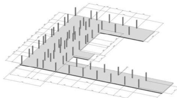
Figure 7. 3D view of the Structural Model is composed of 63 cylindrical concrete columns and one large floor slab.
