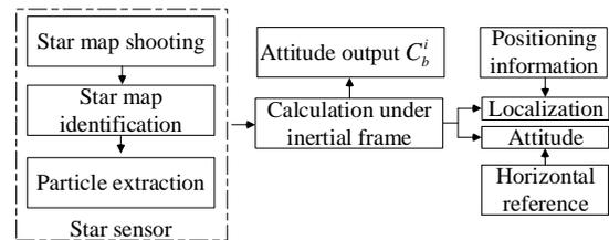
Fig. 3. Principle schematic diagram of the Star sensor
