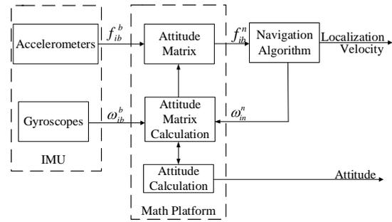
Fig. 2. Principle schematic of the Inertial Navigation System
