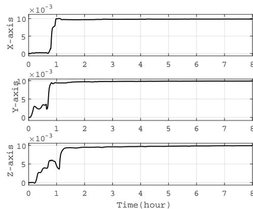
Fig. 5. Estimation results of the gyroscopes' constant bias
