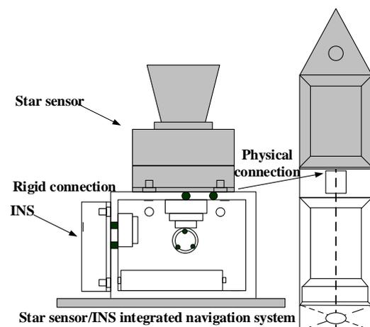
Fig. 4. Installation diagram of the Star sensor/INS integrated navigation system
