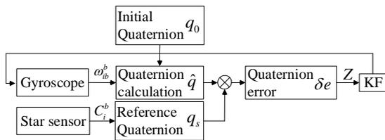
Fig. 1. On-line calibration schematic of the Star sensor/INS integrated navigation system
