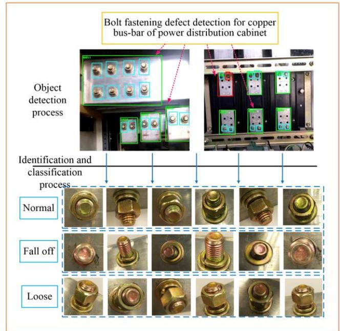
Fig. 5. Visual diagram of bolt fastening defect detection for copper bus-bar of power distribution cabinet.
