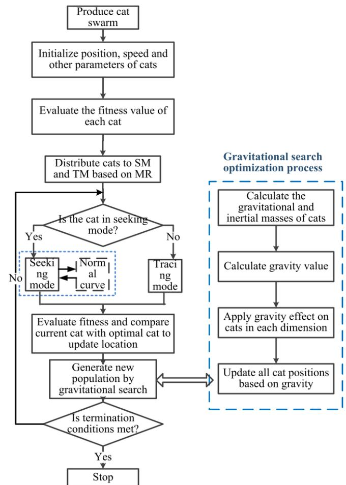
Fig. 3. The GS-NMCSO operation process flowchart.
