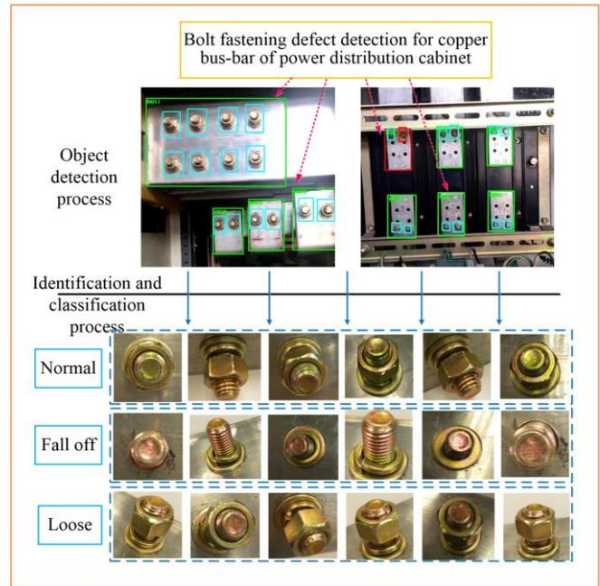
Fig. 5. Visual diagram of bolt fastening defect detection for copper bus-bar of power distribution cabinet.
