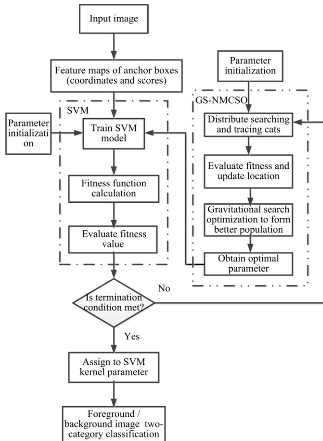
Fig. 4. Parameter optimization process of SVM based on GS-NMCSO.
