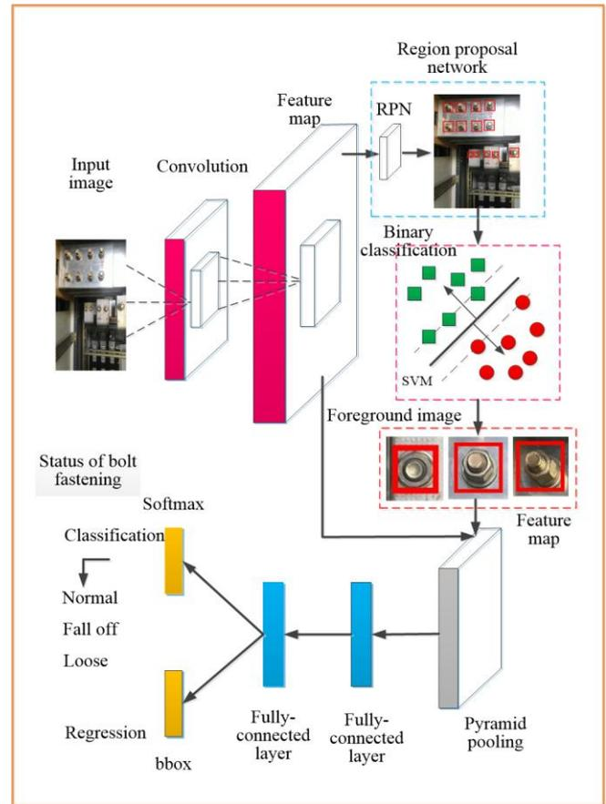
Fig. 2. Optimized cascaded network structure based on SVM.
