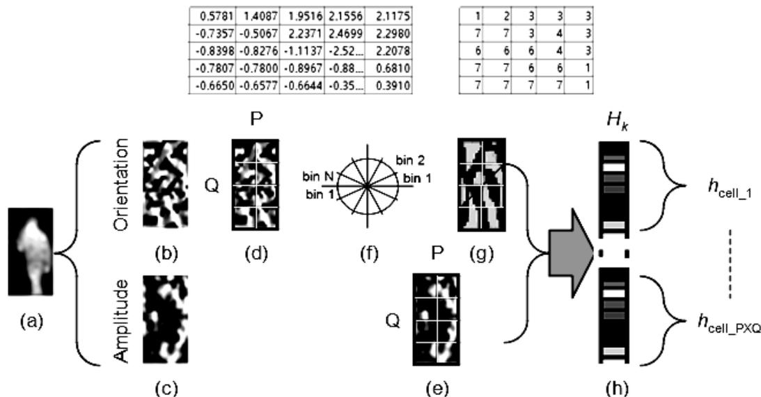
Fig.4. Exemplar images to illustrate the formulation of a feature vector from monogenic components on a specific scale. (a) The ROI; (b)  $\theta_k$  on the  $k$ th scale; (c)  $A_k$  on the  $k$ th scale; (d) cell grids overlapped  $\theta_k$ ; (e) cell grids overlapped  $A_k$ ; (f) setting of directional bins; (g) discrete orientation map; and (h) feature vector that corresponds to the  $k$ th scale.
