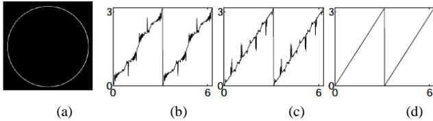
Fig. 1. Orientation estimation of the (b) optimized Sobel operator, (c) SQF and (d) MMSR on (a) the circle image.
