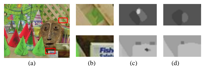
Fig. 4. Disparity map based on color and depth information. (a) Cones test image, (b) intercepting enlarged area, (c) initial method, (d) method using depth information component.
