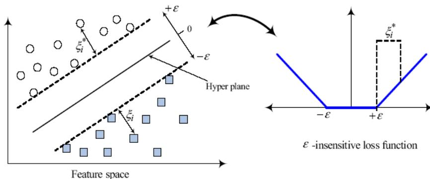
Fig. 1. Transformation process for a SVM regression model.
