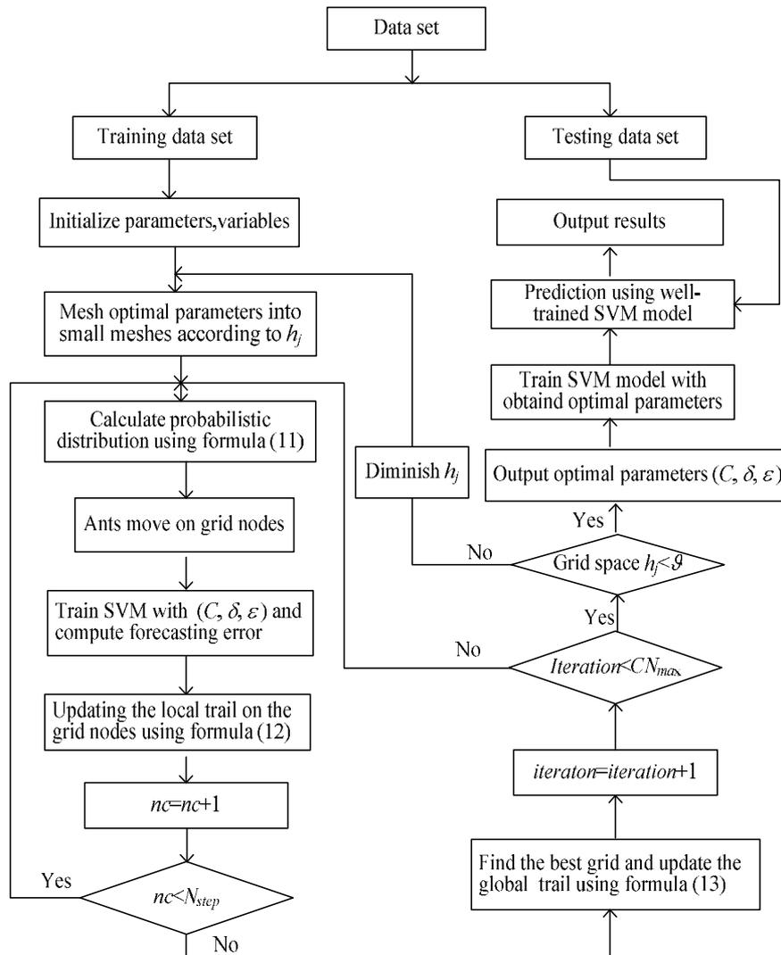
Fig. 3. The flowchart of ACO&SVM model.
