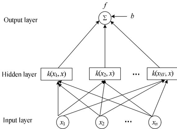
Fig. 2. SVM regression prediction based on phase space reconstruction.
