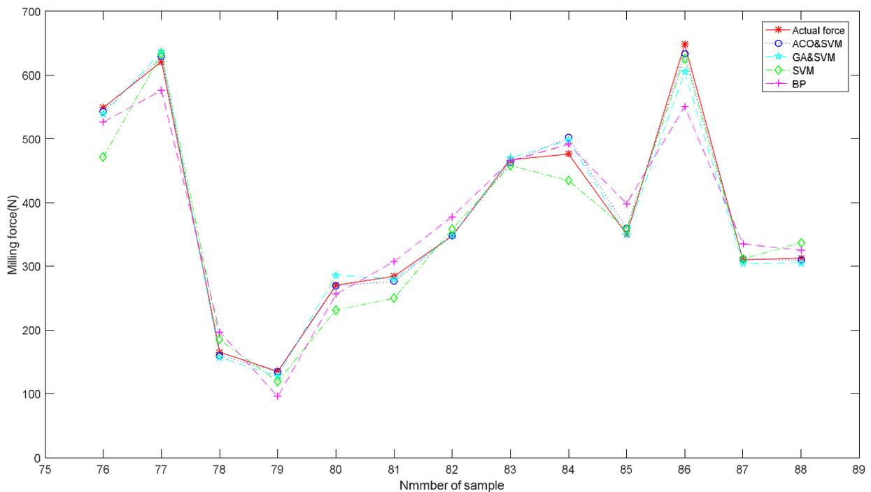
Fig. 8. The actual values of milling force and the forecasting values of four models.
