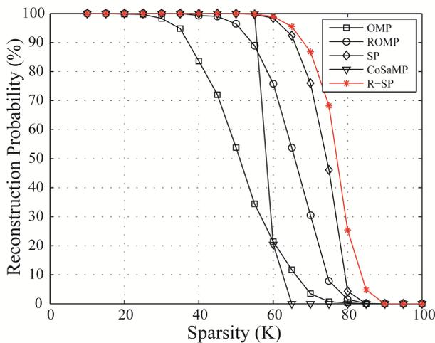
Fig. 4. Simulation curves of reconstruction probability versus sparsity  $K$  when observation dimension  $M = 160$ .
