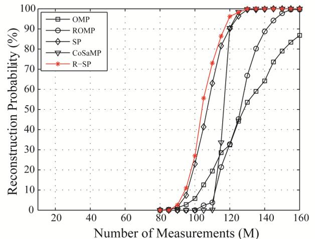
Fig. 2. Simulation curves of reconstruction probability versus the number of measurements when sparsity  $K=40$ .
