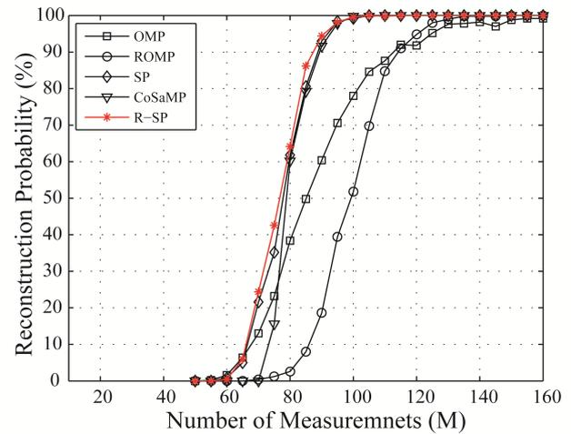
Fig. 1. Simulation curves of reconstruction probability versus the number of measurements when sparsity  $K=25$ .
