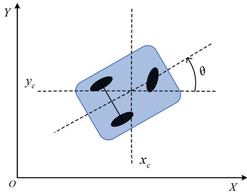
Fig. 1. The planar graph of a mobile robot.
