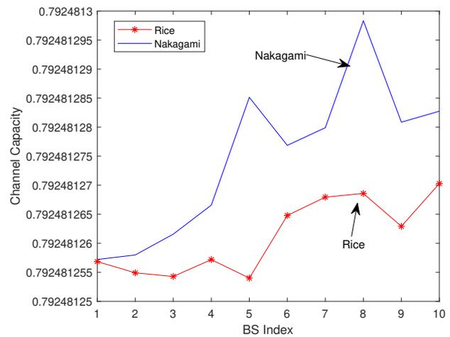
Fig. 3. Channel Capacity of Rice and Nakagami Distribution Channels (bits/s/Hz) vs BS index
