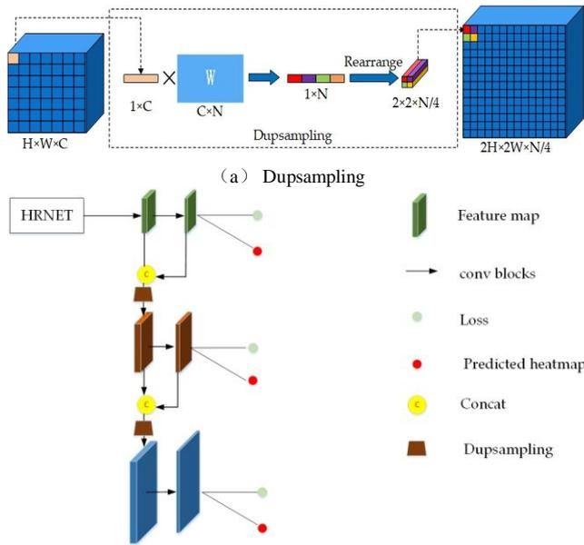
(b) The overall structure of the high-resolution feature pyramid
