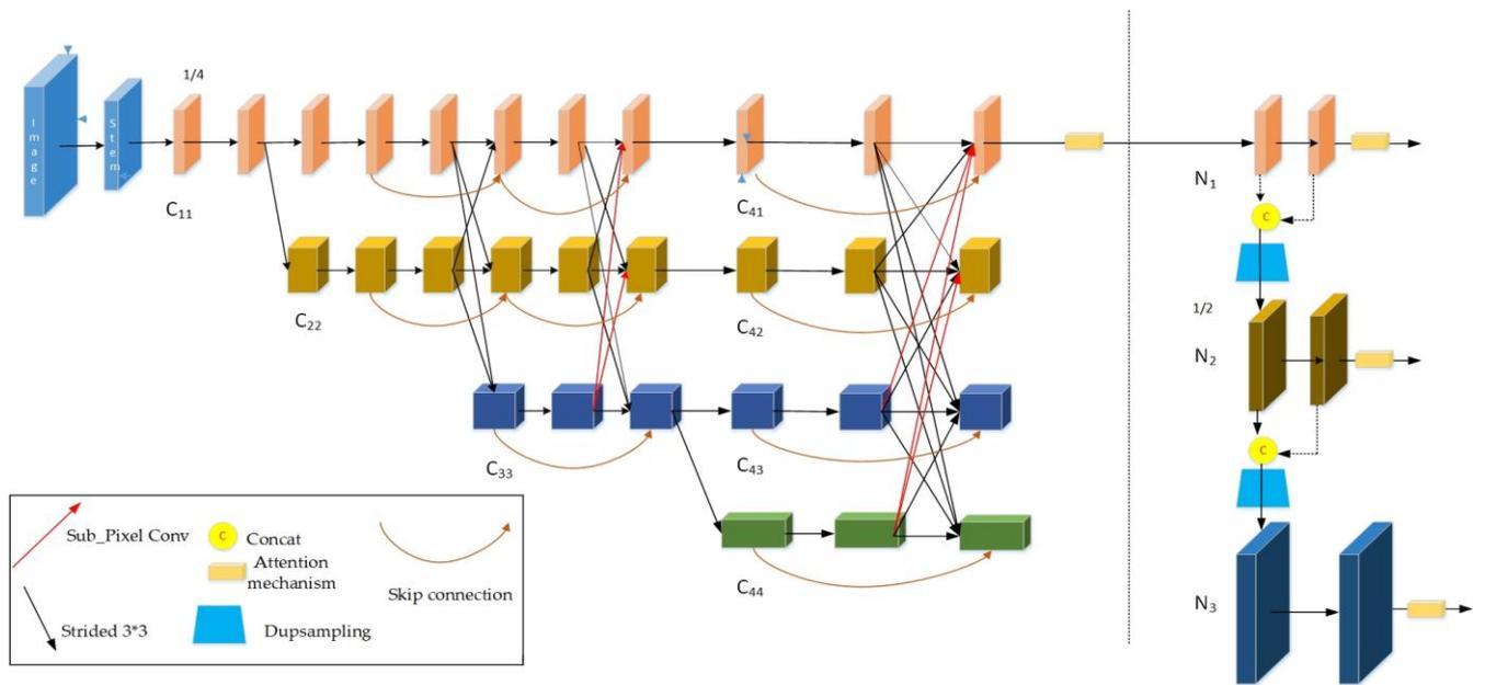
Fig. 2. A schematic of the overall network structure of CE-HigherHRNet. The overall network is composed of an improved backbone and an improved high-resolution feature pyramid.
