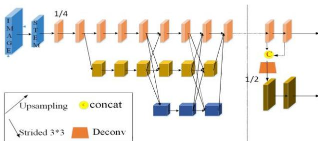
Fig. 1. The original HigherHRNet [5] network structure.
