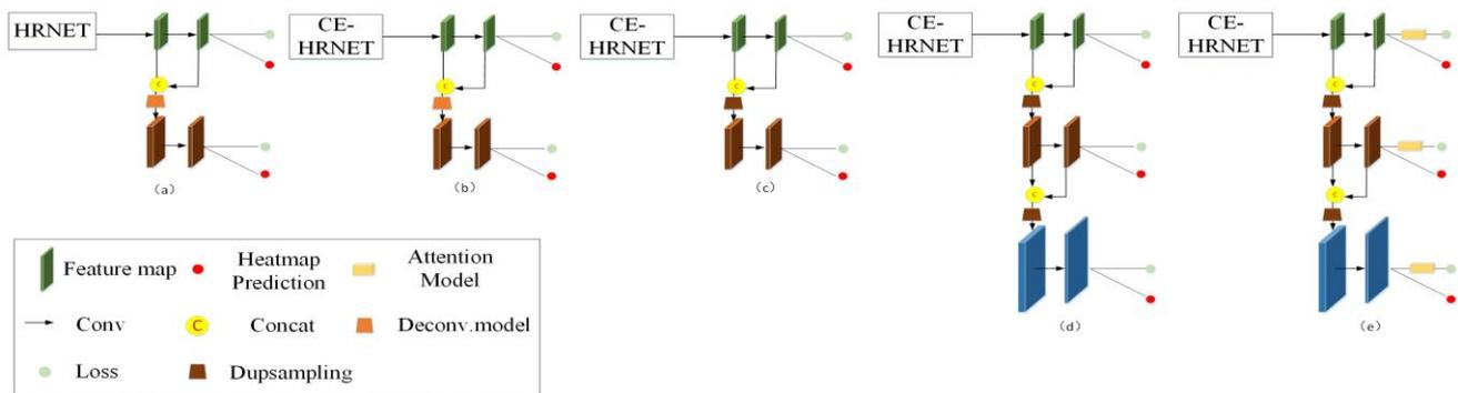
Fig. 6. (a) The original HigherHRNet's high-resolution feature pyramid network. (b) Replace HRNET with the improved CE-HRNET. (c) Use dupsampling module to replace the deconvolutional module to generate feature maps with input image resolution 1/2. (d) On the basis of (c), generate a feature map that is consistent with the resolution of the input image. (e) Add an improved CBAM attention mechanism at the end to form the final network structure.
