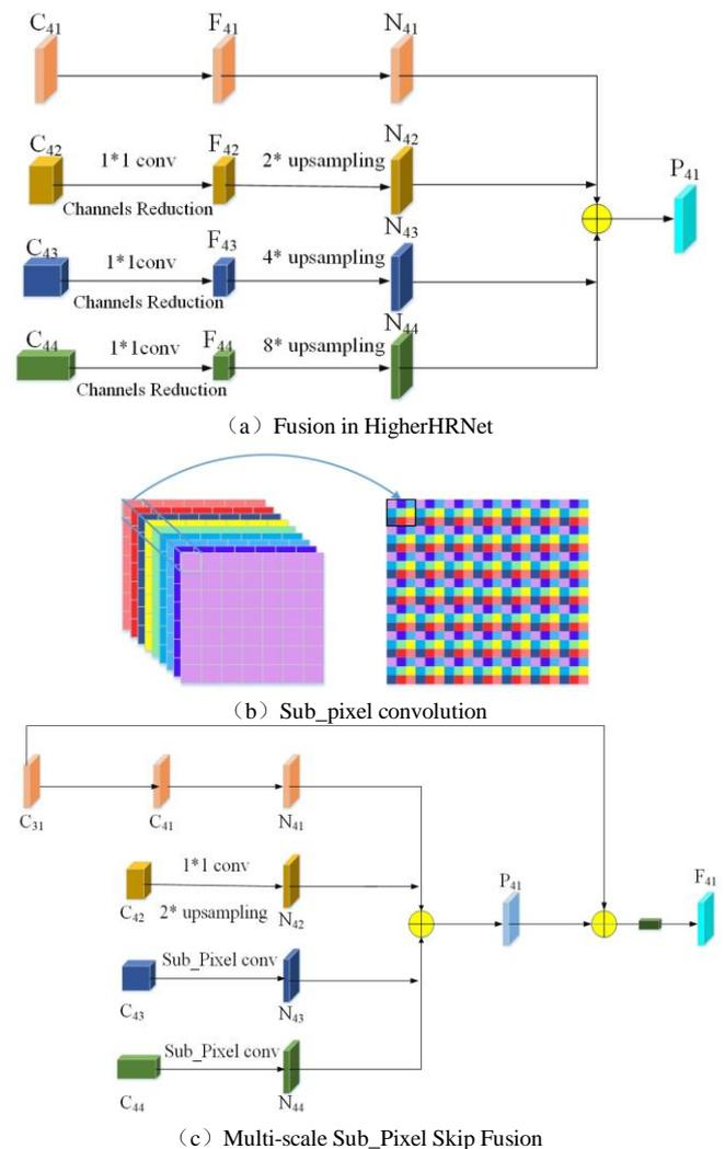
Fig. 3. (a) Shows the fourth stage  $C_4$  fusion method in HigherHRNet. (b) Shows the working principle of Sub\_Pixel, (c) Introduces our Multi-scale.
