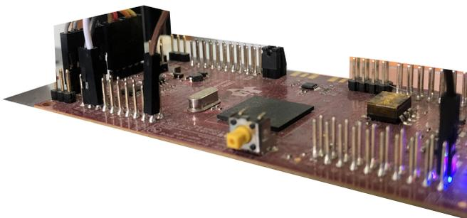
Fig. 5. Texas Instruments F28379d Launchpad connected to the encoders and motor driver.
