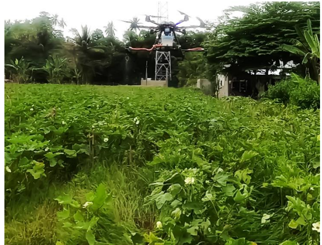
Fig. 1. Vision-based unmanned aerial system sprays at a variable rate over a vegetable field
