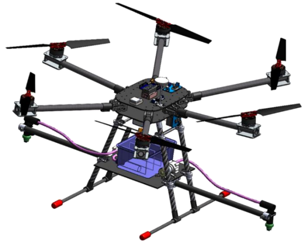
Fig. 5 CAD model of the aerial sprayer system as designed in this study
