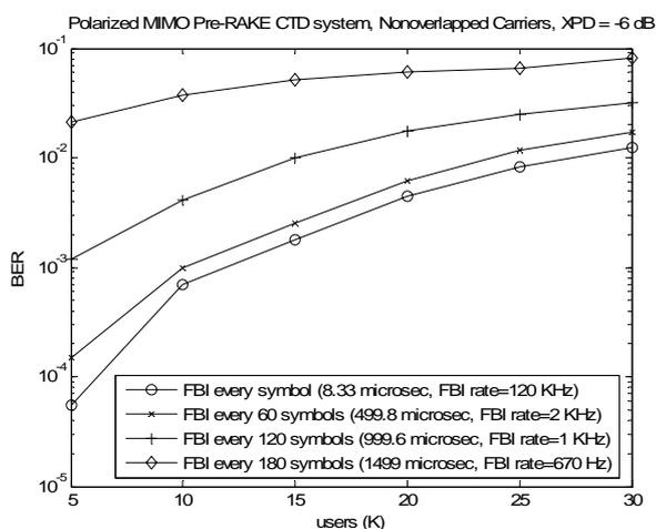
Fig. 8 The performance of the Polarized MIMO Pre-RAKE CTD system using nonoverlapped carriers under different FBI rates,  $E_b/N_o=10$  dB.
