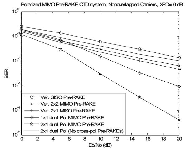
Fig. 5 A performance comparison between the Polarized MIMO Pre-RAKE CTD using nonoverlapped carriers and the Vertical MIMO Pre-RAKE CTD systems when  $K=10$ ,  $L_r=L=3$  and FBI rate=1 KHz.
