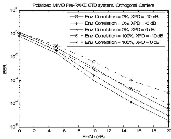
Fig. 7 The performance of the Polarized MIMO Pre-RAKE CTD system using orthogonal carriers under different values of XPD and  $\rho_{env}$ .
