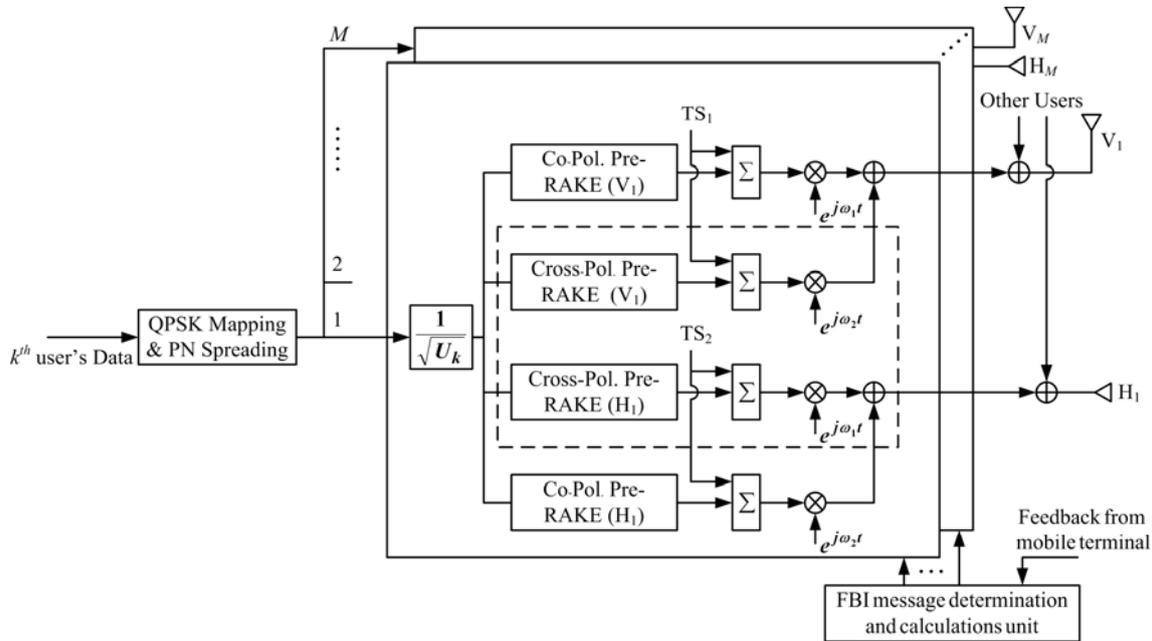
Fig. 1 The Polarized MIMO Pre-RAKE CTD transmitter of the Node B.
