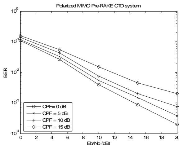
Fig. 10 The impact of the imbalance in the co-pol power intensities (CPF) on the BER performance of the Polarized MIMO Pre-RAKE CTD system.
