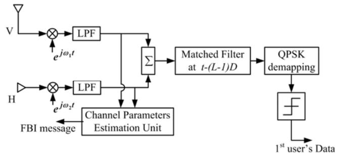
Fig. 2 The Polarized MIMO Pre-RAKE CTD receiver of the 1<sup>st</sup> user's mobile terminal.
