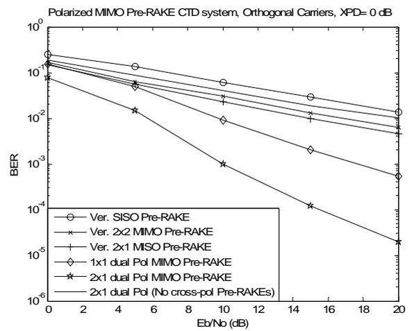
Fig. 6 A performance comparison between the Polarized MIMO Pre-RAKE CTD using orthogonal carriers and the Vertical MIMO Pre-RAKE CTD systems when  $K=10$ ,  $L_r=L=3$  and FBI rate=1 KHz.
