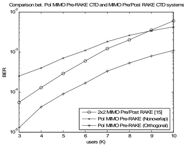
Fig. 4 A performance comparison between the Polarized MIMO Pre-RAKE CTD and the Pre/Post MIMO CTD systems when  $E_b/N_o=8$  dB,  $N=8$  and  $L_r=L=2$ .
