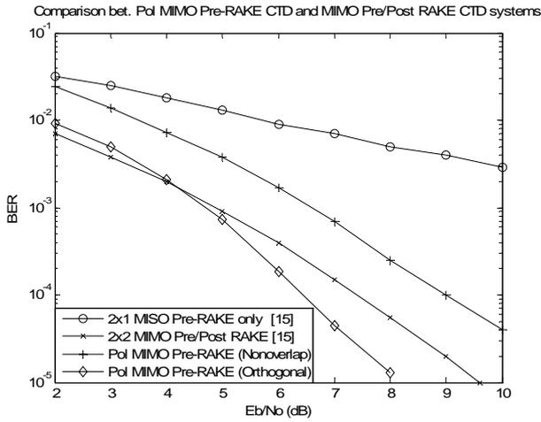
Fig. 3 A performance comparison between the Polarized MIMO Pre-RAKE CTD and the Pre/Post MIMO CTD systems when  $K=3$ ,  $N=8$  and  $L_r=L=2$ .
