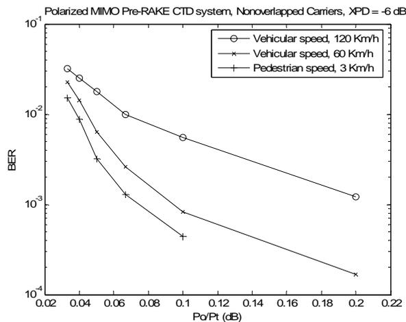
Fig. 9 The performance of the Polarized MIMO Pre-RAKE CTD system using nonoverlapped carriers for both vehicular and pedestrian speeds,  $E_b/N_o=10$  dB.
