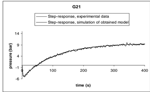
Fig.6 Comparison of  $G_{21}$  simulated step-response with the experimental result.
