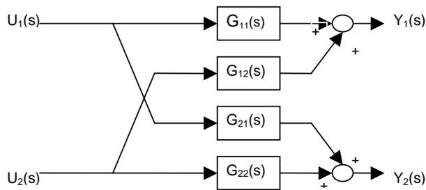
Fig. 3 Input-output model of the system
