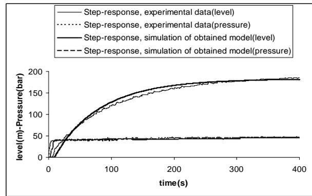
Fig.7. Comparison of simulated system models and experimental unit-step responses
