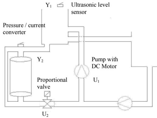
Fig. 2 Block diagram of the pressure-level system
