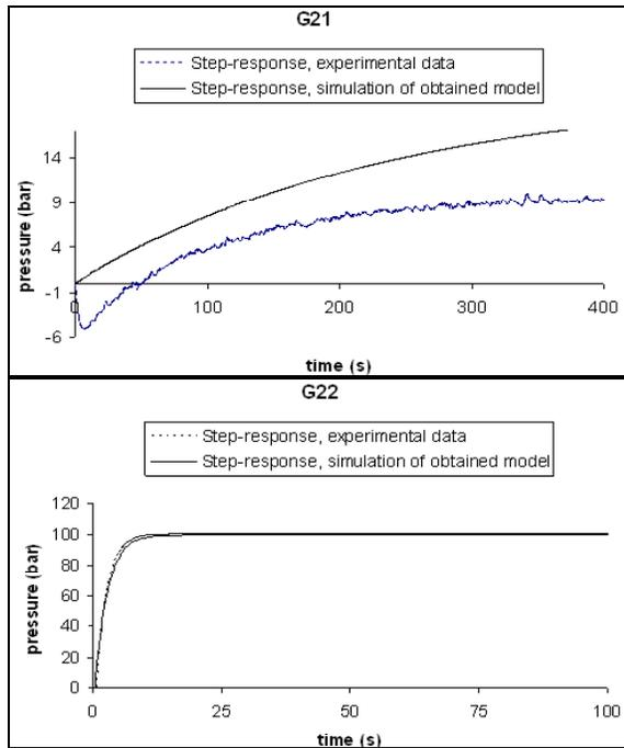
Fig.5 Comparison of experimental step-responses and transfer functions obtained by real-time identification
