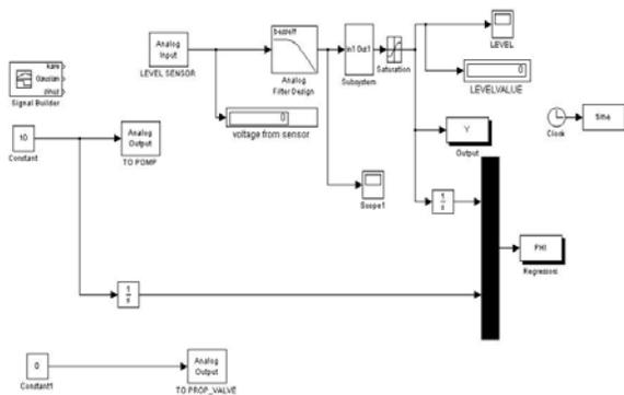
Fig. 4 MATLAB interface for real-time system modeling
