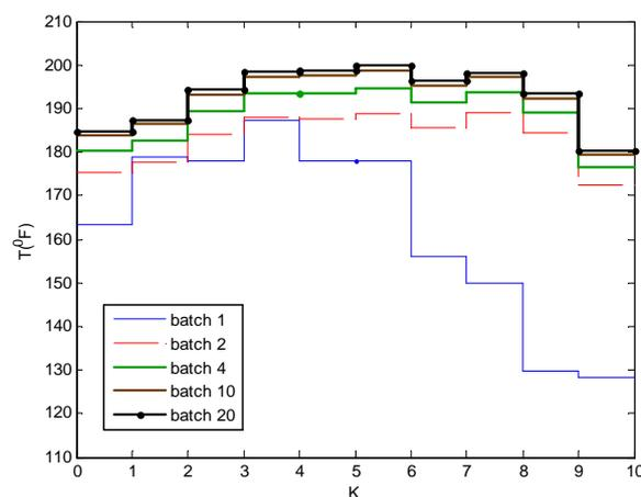
Fig. 5. The evolution of the designed temperature trajectories for the setpoint change using the two-step MPLS based ILC
