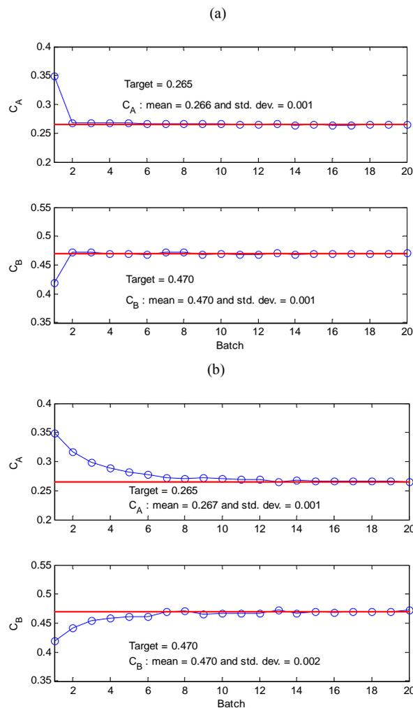
Fig. 4 Convergence of  $C_A$  and  $C_B$  for the setpoint change using (a) the two-step MPLS based ILC; (b) the standard MPLS based ILC.
