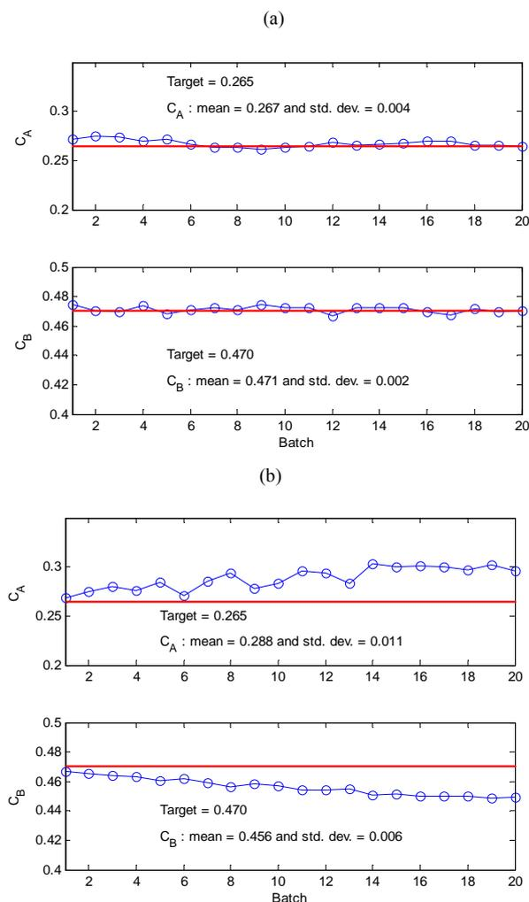
Fig. 5 Convergence of  $C_A$  and  $C_B$  for the disturbance change: (a) with the update of the two-step MPLS models, (b) without the update of the two-step MPLS models.
