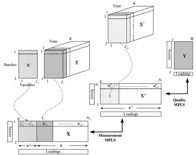
Fig. 1. Data structure for modeling a batch process.
