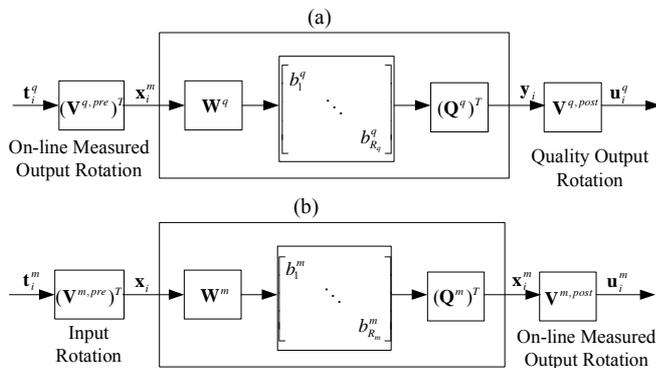
Fig. 2. Diagonalize the batch process: (a) on-line measured outputs and quality outputs; (b) inputs and on-line measured outputs.
