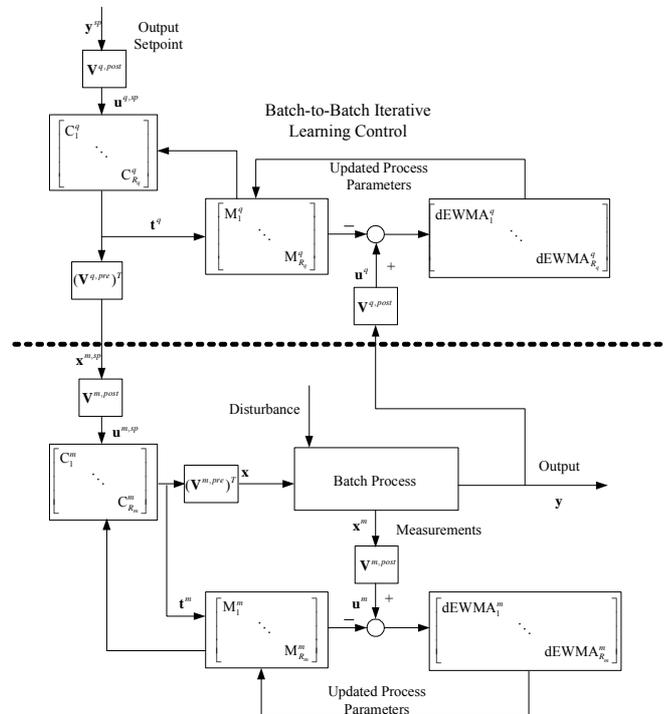
Fig. 3. The structure ILC design using two-step MPLS models.
