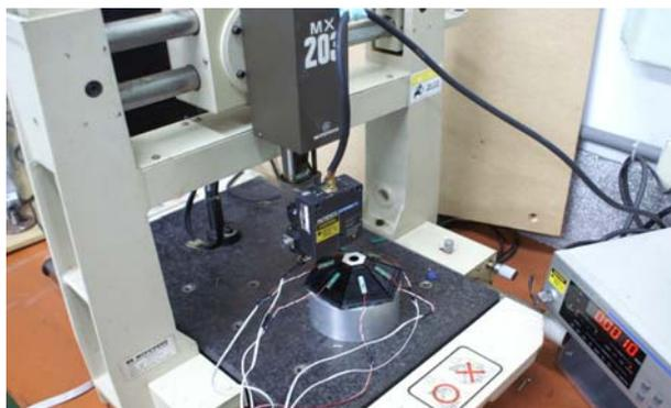
Fig. 11 The six-axis stages in experiment
