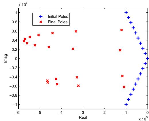
Figure 5: Initial pole placement and final pole locations in Example 2.
