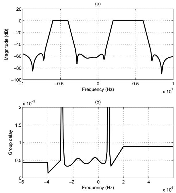
Figure 4: Frequency response of Example 2. (a) Magnitude, (b) Group delay in passband.
