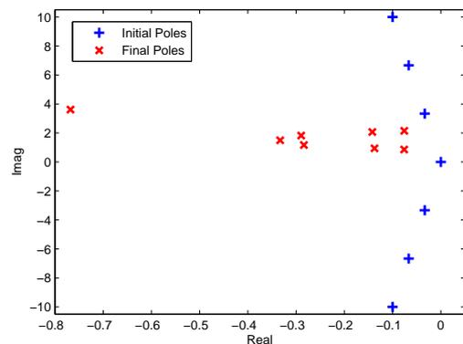
Figure 3: Initial pole placement and final pole locations in Example 1.
