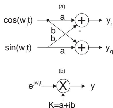
Figure 1: (a) The real signal-flow graph (SFG) of a complex multiply and (b) the equivalent complex SFG.
