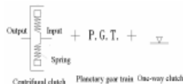
Figure 9 Concept of the invention of automatic transmission
