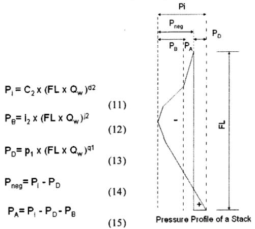
Figure 3 Computation approach of the NTUST simulation model
