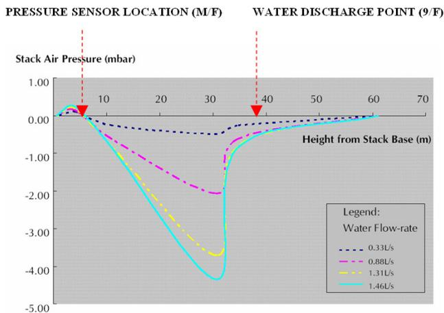
Figure 9 Air Pressure profile in Stack at Block M
