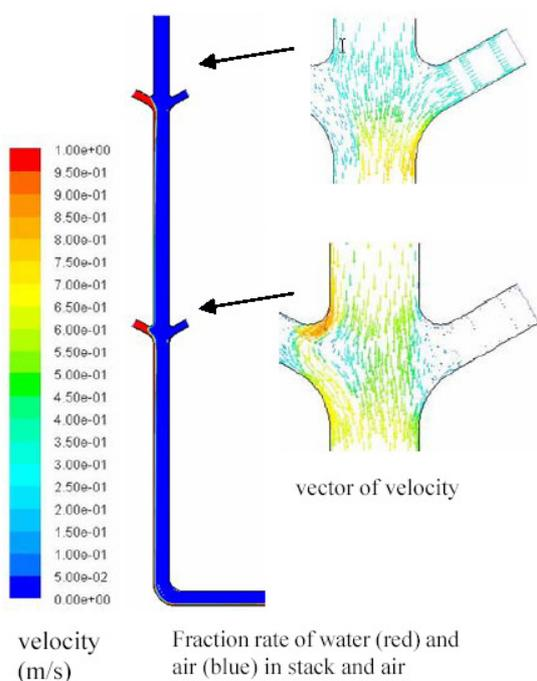
Figure 6 CFD simulation result
