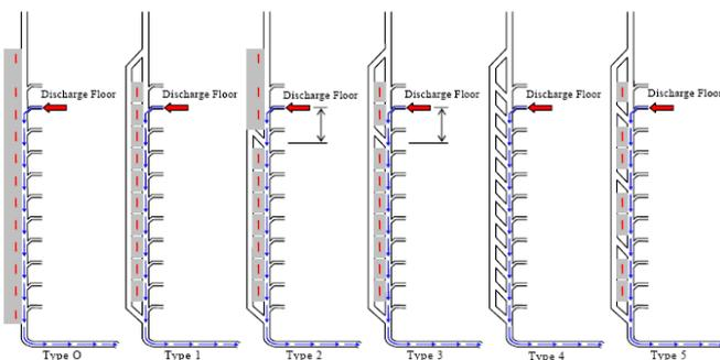
Figure 4 Different ventilation conditions in the NTUST model
