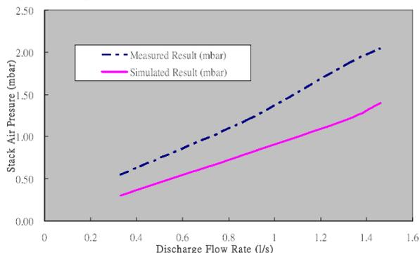
Figure 10 A comparison on the air pressure transient propagation between observed and simulated results at the measurement point (M/F)
