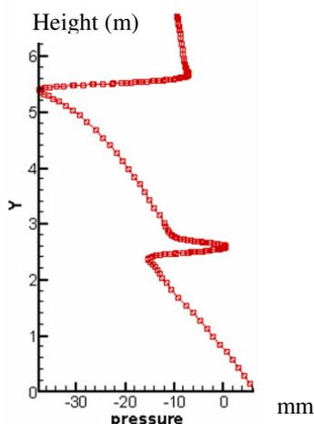
Figure 7 pressure profile of stack
