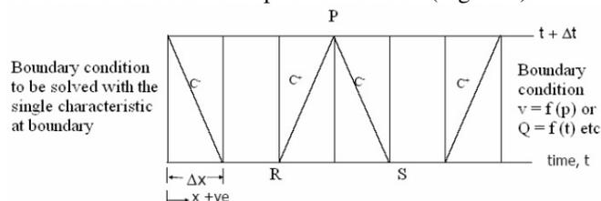
Figure 2 Set up C+ and C- equations and solve by different boundary conditions.
