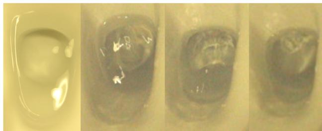
Figure 11 Trap seal oscillation (from a stationary state to the establishment of air bubble path)
